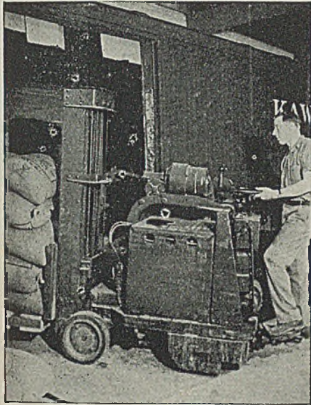
Forked truck loading bagged materials into a railroad freight car. One man handles the work of many.
