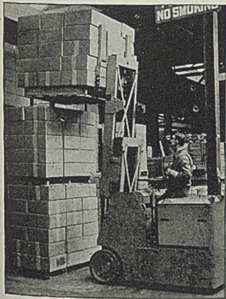
Forked truck stacking palletized unit load. This method doubles storage capacity of warehouses.
