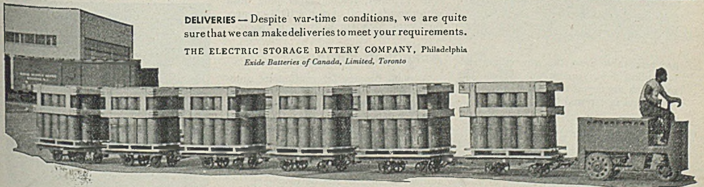
Tractor-trailers speed-up loading operations. Palletized loads can be placed on trailers by forked trucks, hauled to storage or shipping points and unloaded by forked trucks for additional speed and prevention of materials-damage.
