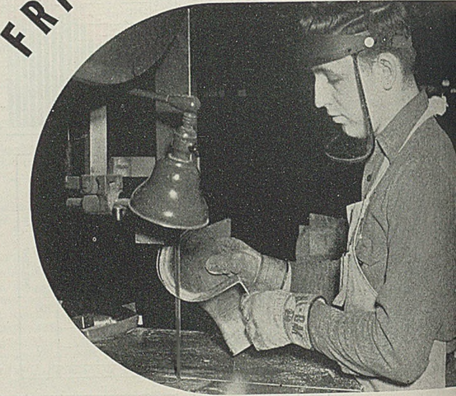
Fig. 1—Friction process is especially advantageous for cutting pieces of odd shape which the operator may manipulate freely as in the case of the aircraft part shown here. The saw runs at 12,000 feet per minute against 100 to 500 for usual metal cutting
