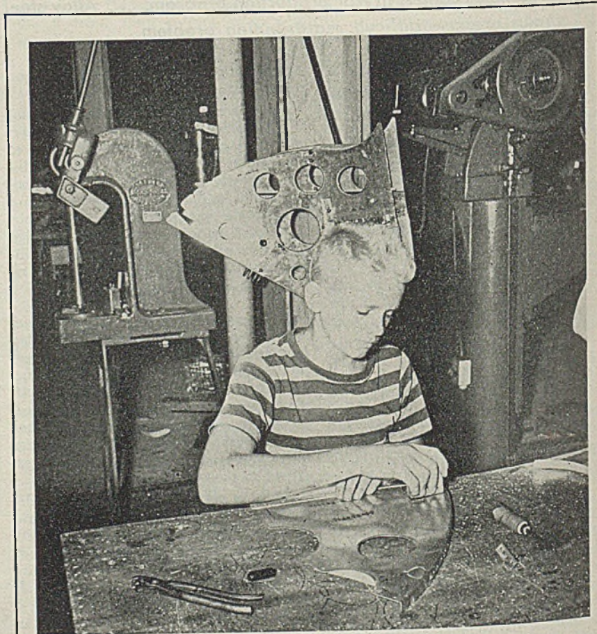
BOYPOWER: Sixteen hundred Akron high school students are working a half shift before or after school at the Goodyear Aircraft factory. Youth shown above removing burrs from a bomber section is one of hundreds enrolled in the company's apprentice mechanics' course
