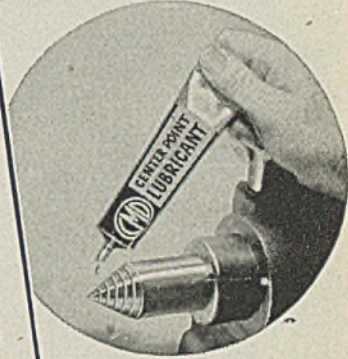
The center shown above is the famous CMD Helical Groove Center which has a left-hand helical groove that conveys the oil constantly to the extreme point of the center.
