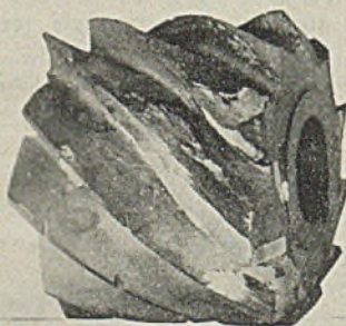
Same Slab mill as reclaimed by "SUTTONIZING." Also rough ground.
