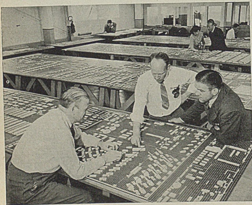
Boeing engineers "play chess" with wood blocks representing machine units in the vast machine shop at the new Boeing plant at Renton, Wash. Every piece of equipment in the plant, from wing jigs to the smallest parts bin, is duplicated on the planners' boards
