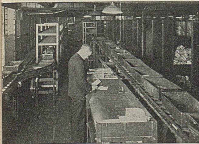
Fig. 4 (Right below)—Work comes to this drill press group on upper level of conveyors, is returned to central station when completed by placing on lower conveyor level. Fully automatic
