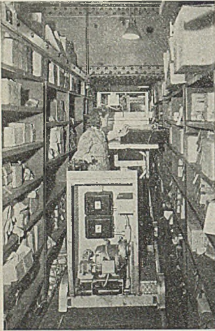
Fig. 5 (Left)—Special car facilitates storeroom operations in aisles 60 feet long
