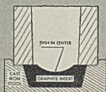
Carbon or graphite stool insert with dish surface. Replacing copper.
