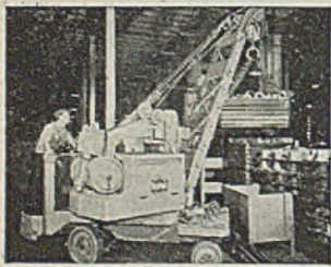
Small parts in standard boxes are tiered by Baker Truck to conserve space.
