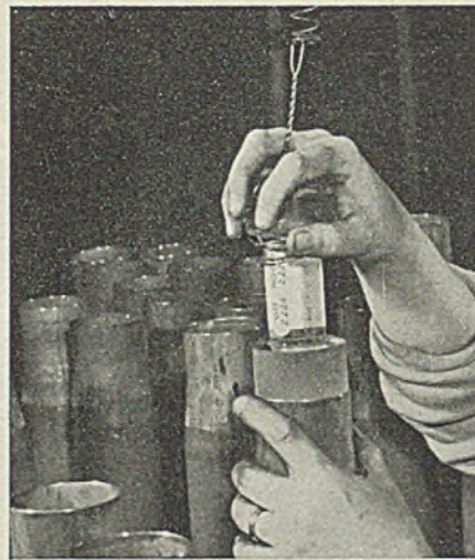
Fig. 16—A glass gage being used to check inside diameter of cartridge cases. Neither ductility nor impact resistance is required in this service 4b . Official OWI photo
