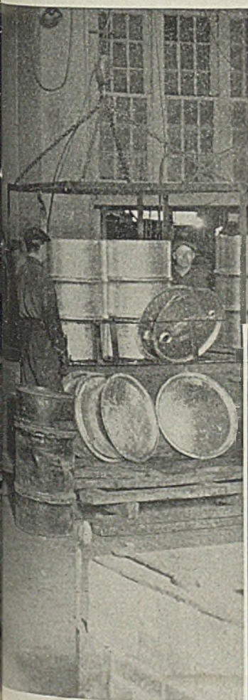
(Right)—U. S. Navy ammunition container shown here is drawn from steel, zinc plated and chromated. The container is 6\frac{3}{4} inches in diameter and 31\frac{1}{2} inches long
