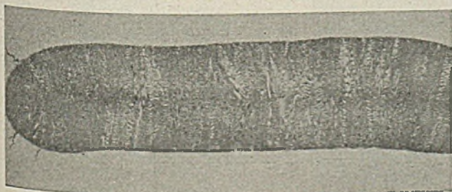
Fig. 6—Typical weld, 0.062-inch sheet, at recommended welding conditions; left, one end of weld nugget; right, portion of weld center at 100 diameters
