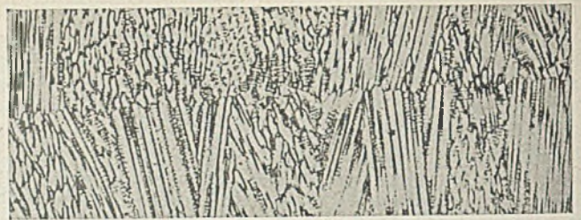
Fig. 7—Typical weld in Inconel 0.062-inch sheet at recommended welding conditions; left, at 12 diameters, shows one end of weld nugget; right at 100 diameters is portion of weld at center
