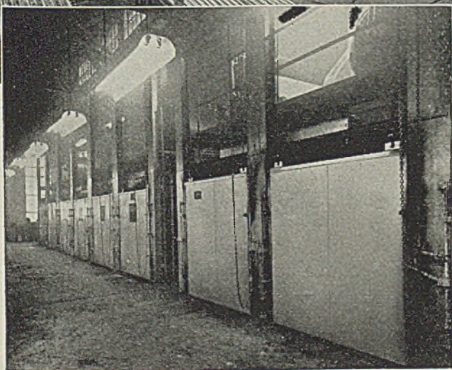
Above: 8 of the many Maehler core ovens at Howard magnesium, aluminum and bronze foundries.
