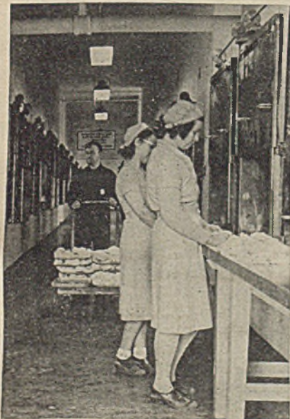
Routing filled bags to packing department. Corridor of a bag loading house. Girls check bags and push them through chute
