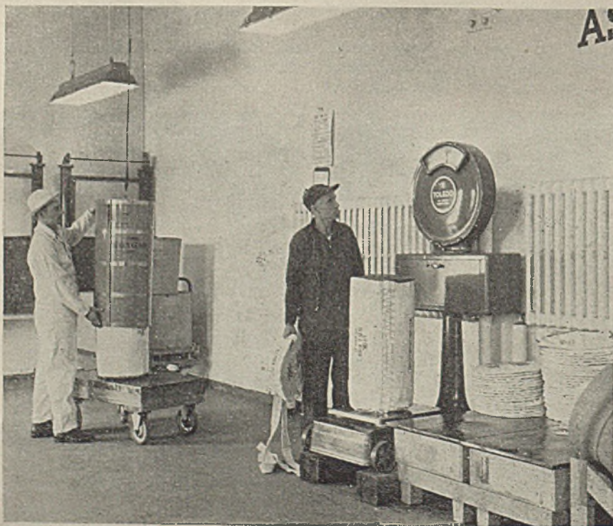
Gaging and weighing powder charges for 16-in. cannon. Note the new explosion-proof fixtures for protection of the fluorescent lights. Safety precautions to prevent sparks are exceedingly thorough
