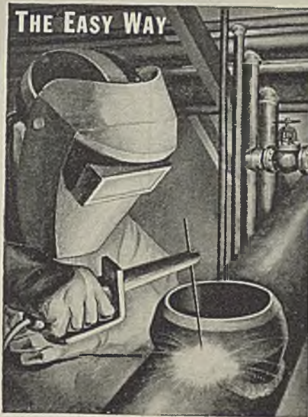
With W-T's* you simply select the position of the outlet on the main pipe and weld the fitting into place, either before or after erection of the main line. The hole is usually cut in the main pipe with the torch after the fitting is installed.
