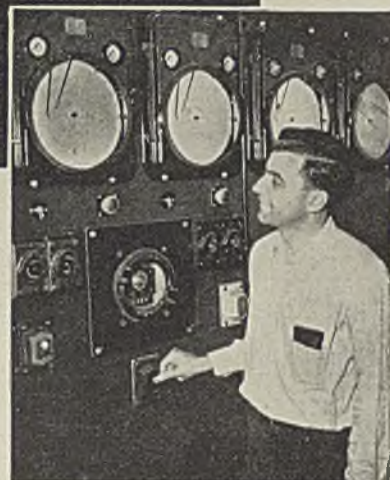
Pushing a tiny button, the operator of the control board activates the Bristol instruments which started production of synthetic rubber in the United States Rubber Company's New England plant.
