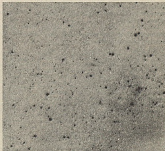
FIGURE 3. MICROPHOTOGRAPHIC DETAIL FROM LEAD PATTERN OF SECTION OF BRONZE, \times 20
