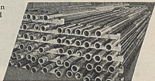
A Few of the 236 Brown Fintubes used in 2 Toluene Plants, Tubes, 6" OD, ¾" Wall, 36' Long 9% Chrome Steel. Fins, 4-6% Chrome Steel.
