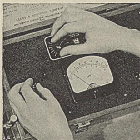
Electrode calibration is compensated by a second knob. Only the temperature compensator need be reset for later tests.
