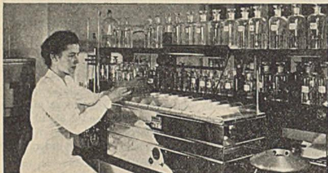
When these covers were put to use, moisture condensed on the inside, reached the saturation point, then abruptly ran down to the lower edges of the covers and dropped off into the water bath, instead of onto the test tubes, as with metal covers.
