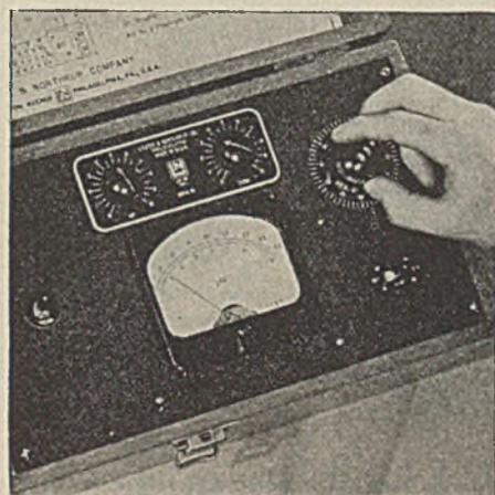
Manual temperature compensator, set to solution temperature, eliminates computations, thus saving time and avoiding errors.
