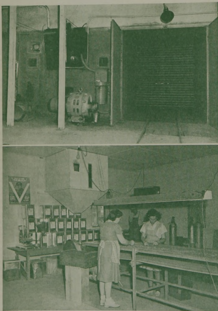
Courtesy, E. A. Couture Company Dehydrating Tunnel for Carrots (above); Sorting Dehydrated Carrots to Be Sealed in the 5-Gallon Cans Shown at the Left (below)
