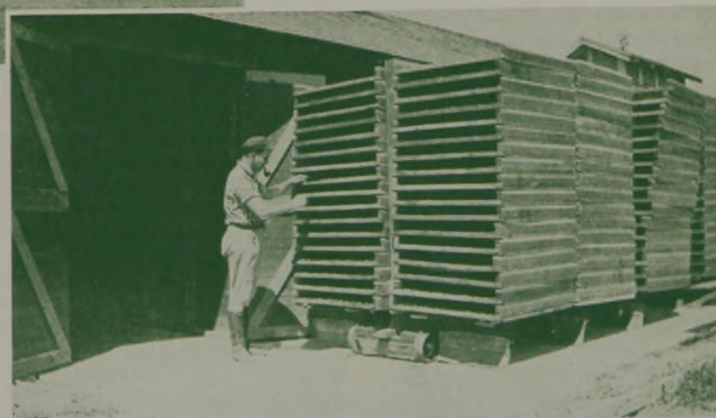
The Center Picture Shows Racks of Dehydrated Potatoes Laid Out in Trays Similar to the Two Shown at the Top; Below Are Several Large Potato Dehydration Tunnels in California
