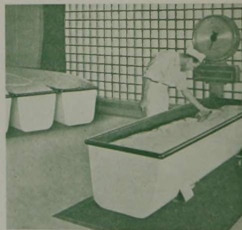
Weighing and Taking the Temperature of a Dough in the Fermentation Room
