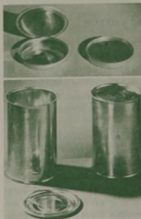
(Above) Thermal Death Time Cans (2 1 / 2 Inches in Diameter, 3/8 Inch High), Open and Assembled
