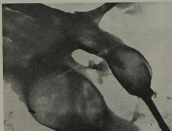
FIGURE 2 (Top). EDGE OF UNFIBRILATED 15-DAY COTTON FIBER ( \times 7500 ); LONGITUDINAL STRIATION IS APPARENT
