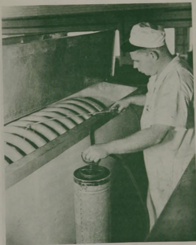
Spraying Previously Cleansed Coil Pasteurizer Vat with Acid Cleaner Solution (Replacing Chlorine Rinse Solution) to Prevent Contamination by Quality-Defective Microorganisms
