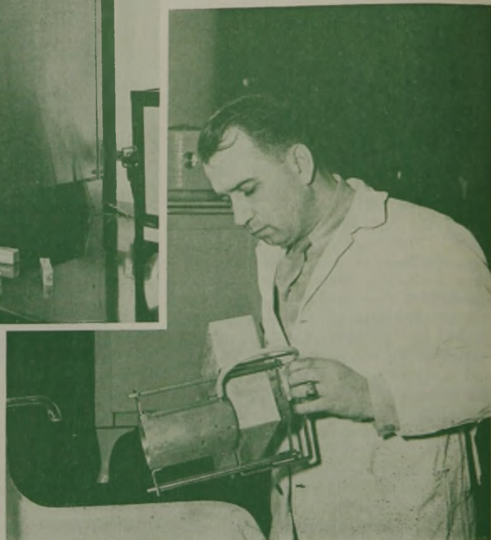
(Below) Checking the Tightness of a Sealed Wax Wrapped Carton
