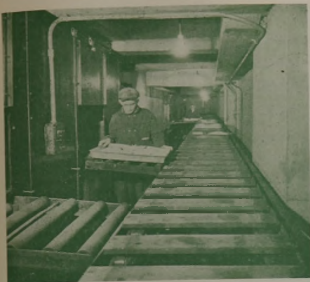
Courtesy, Commonwealth Ice and Cold Storage Company Conveying Fish by Pan Elevators from Panning Room to Sharp Freezers
