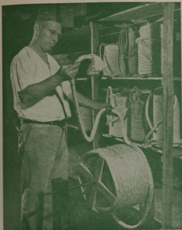
★ Square - Braided Packing, Made from Continuous Filament Rayon "Tow", Is Serving War Industry in Water Pumps, Accumulators of Hydraulic Presses, Punches, Etc., Where It Replaces Packing Made of Imported Long-Line Flax
