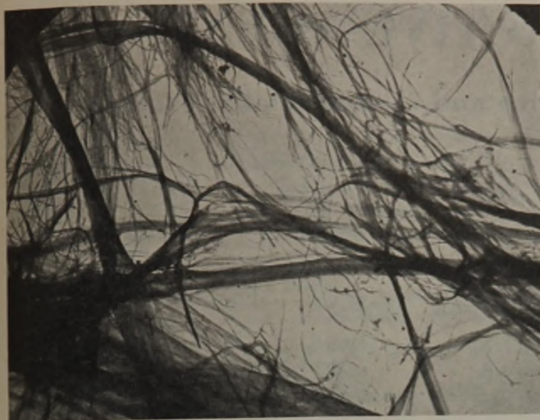
FIGURE 7. FILTER PAPER (WHATMAN'S GRADE 0) MECHANICALLY DISINTEGRATED IN WATER ( \times 6000 )
