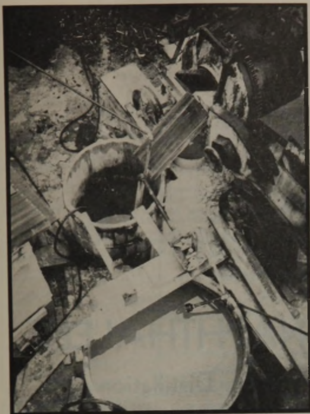
Figure 2. Pilot Plant for Chemical Beneficiation of Celestite-Strontianite Ore
