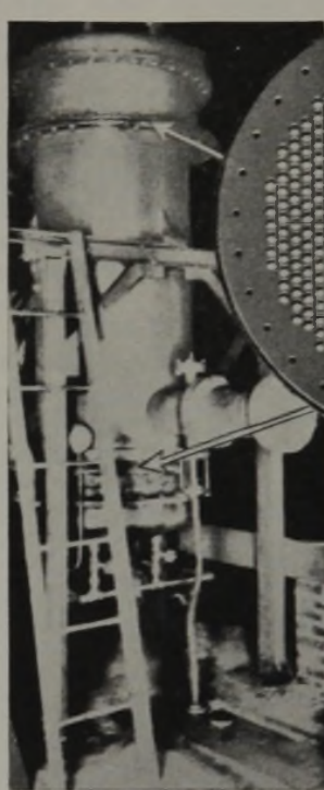
Ace rubber lined chlorine gas cooler, equipped top and bottom with Ace rub- ber covered tube sheets. Sheets have 673, 13/16 inch diameter holes accu- rately reamed.
