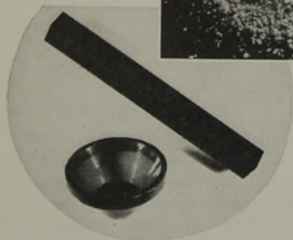
FIGURE 2. BAR AND SMALL CUP MOLDED FROM CORNSTARCH TRIPROPIONATE, PLASTICIZED WITH 10 PER CENT DIBUTYL PHTHALATE
