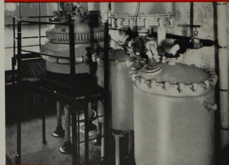
FULL SCALE Glass-lined reaction kettles are built larger, for higher temperatures and pressures than ever before.
