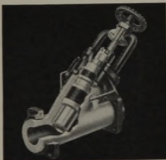
The Lapp Valve is designed to bring liquids into contact only with porcelain. Fine grinding, polishing and lapping of bearing surfaces—and a unique spring washer arrangement—assure smooth action, and a permanently maintained seal, even under vibration and thermal change.
