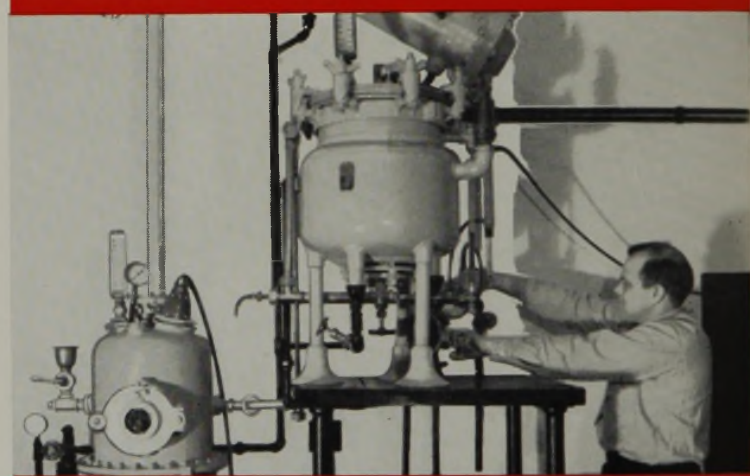
SEMI-WORKS New "P" Series reaction kettles range from 5 gallons up, built for high pressure work.
