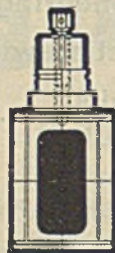
4" Cylindrical Plug of A.C.F. Valve: Area 12.73 sq. in., full pipe area port opening!
