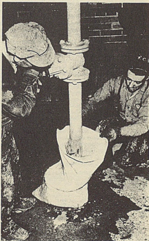
Thiokol Emerges from the Storage Tank, in a Water Carrier, in the Form of Floc; Water Seeps from the Bag Leaving the Floc Ready for the Next Process
