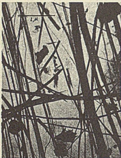
Figure 29. Portland Cement A Hydrated One Week ( \times 16,500 )
