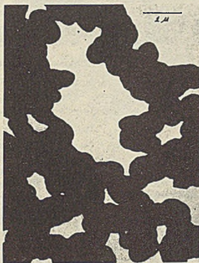
Figure 15. Tricalcium Silicate Hydrated 10 Days ( \times 10,500 )
