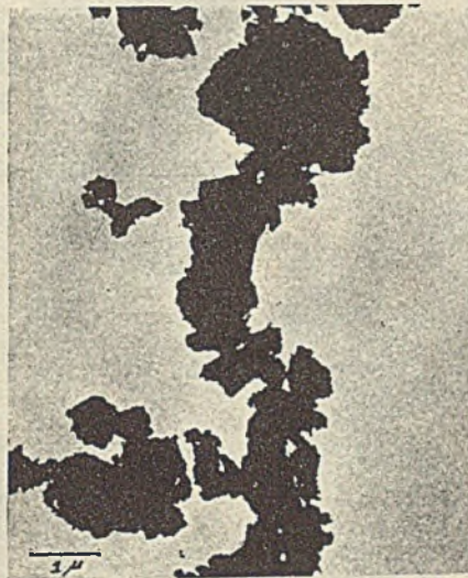
Figure 2. Neat Cement Pat, Ground in Mortar and Dispersed in Petroleum Ether ( \times 8000 )
