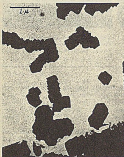
Figure 14. Tricalcium Silicate Hydrated 10 Days ( \times 13,500 )
