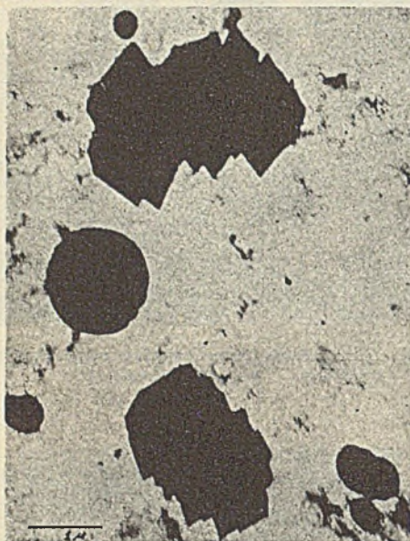
Figure 20. Tricalcium Aluminate Hydrated 10 Days ( \times 10,500 )
