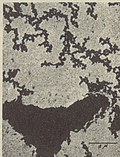
Figure 16. Tricalcium Silicate Hydrated 2 Hours ( \times 12,500 )
