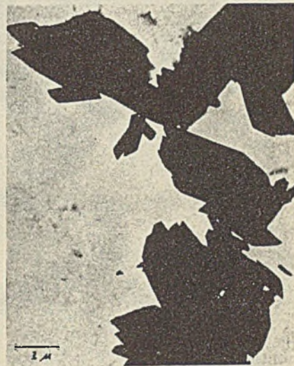
Figure 3. Calcium Sulfate Hydrated 18 Hours ( \times 8000 )
