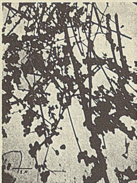
Figure 26. Tricalcium Aluminate (4 Parts) and Calcium Sulfate (1 Part) Hydrated 10 Days ( \times 8000 )
