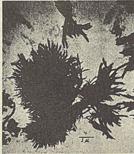
Figure 7. Calcium Hydroxide Hydrated 7 Days ( \times 6000 )
