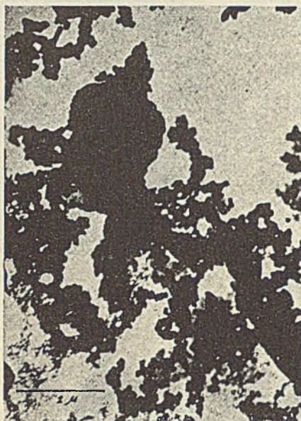
Figure 21. Tricalcium Aluminate Hydrated 10 Days ( \times 16,500 )
