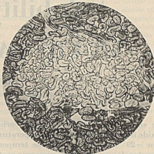
Figure 2. Cotton Fibers ( \times 250 ) after Being Treated With Solution of Copper Salt, Washed Free of Excess Copper, and Placed in Potassium Ferrocyanide Solution
