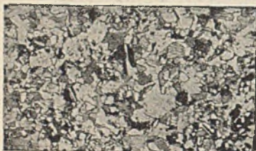
Photomicrograph of weld zone, showing grain structure of weld and parent metal.
