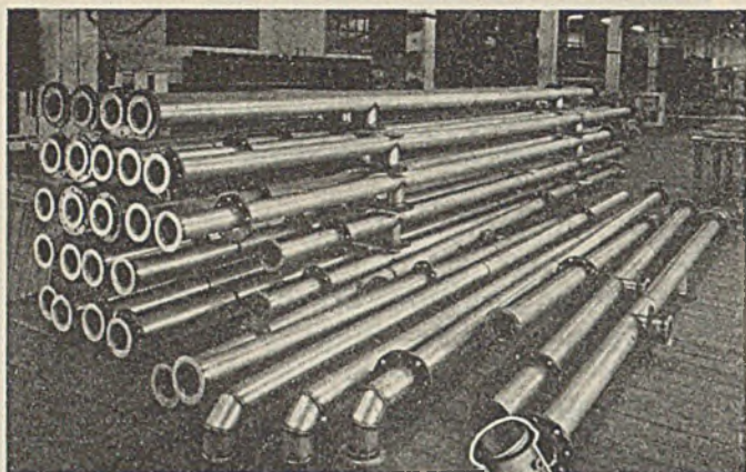
Stainless steel welded process piping with built-up Van Stone joints. PLATE No. 7079
