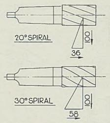
Fig. 8—Comparative pull-out tendency for 20-degree and 30-degree spirals
