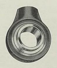
standard Sealmaster seals arranged to form an air-tight chamber which keeps out dirt and retains lubricant. Bearing housings are of Meehanite construction and all but the bronze alloy retainer are specially treated to resist rust. For mounting bearing on shaft, one-half dog-point set screws with lock wires are furnished as standard equipment.
