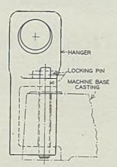
Fig. 1—Diagram of special hanger with locking pin in place on machine base ready to lift
