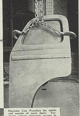
Precision Cast Punches for inside and outside of truck doors. Purchaser reports important savings in weight of metal purchased as well as in time saved through the elimination of profile machining.
