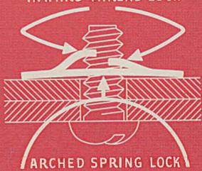
ELIMINATE THREADED NUTS AND LOCK WASHERS
