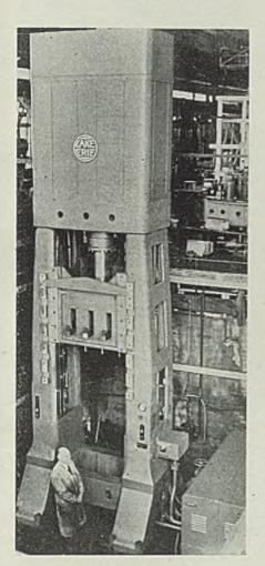
Top of press is completely enclosed in removable panels. High speed pumping unit gives maximum production with fast approach and return of moving platen.
