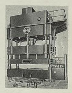
industry. It embodies three separate hydraulic actions for operating, respectively, the main draw punch, the blankholder ring and the die bottom of the regulation triple-action drawing die. The draw punch is carried by the main slide actuated by the main hydraulic press ram of
