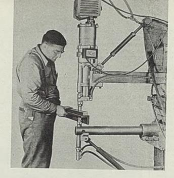
Structural sections are spot welded as easily as sheet metal
