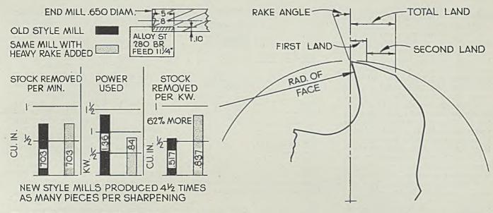
Fig. 3, left, shows remarkable effect of adding heavy rake.
