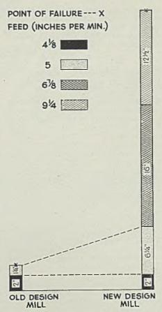
Fig. 11—Graphic comparison of cut taken before failure on old and new type mills. Old mill at failure was cutting at feed of 5 inches per minute against 9½ for new type
