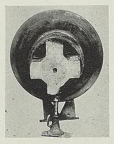
Fig. 4—Roll pod showing the excessive wear that occurs and details of the built-up areas
