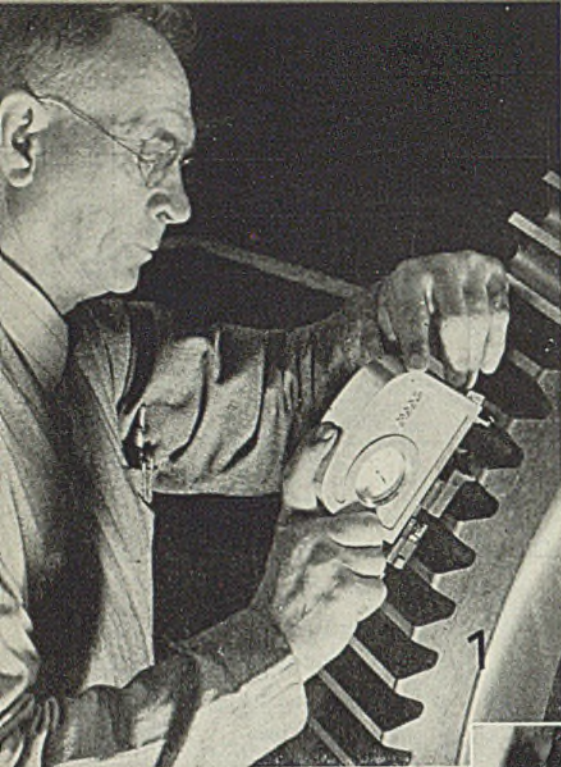
Fig. 1—To obtain quietness of operation at high pitch-line speeds in a gear like this one for a modern locomotive, tooth contours must be true involute curves as nearly as possible. For detailed checking, this unusual Maag instrument is used to measure base or normal pitch at any angle between base and tip
