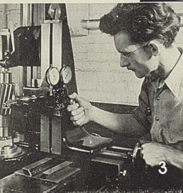
Fig. 3—Checking a finished pinion for correct tooth spacing and tooth profile between centers in a machine with a 3-finger arrangement. One finger is positioned against a given tooth; second finger, spring actuated, provides constant pressure of the pinion against the fixed finger; the third finger actuates the dial indicator which reads deviation from correct spacing between adjacent teeth. A sine bar insures accuracy. Its setting is checked by precision gage blocks. For checking tooth profile, an indicator finger is placed at tooth root and deviation from a true involute read at intervals of 0.015 to 0.020-inch until tooth tip is reached. Tolerance for tooth profile error is 0.0002-inch
