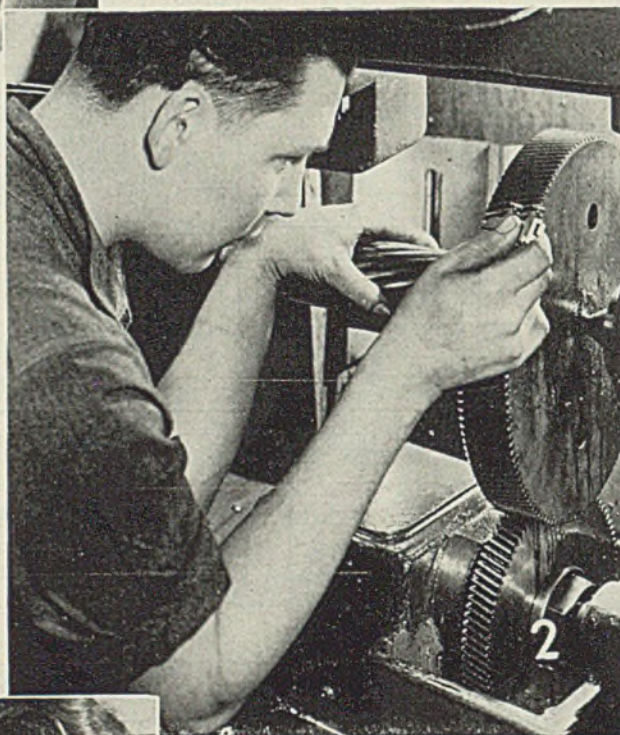
Fig. 3—Checking a finished pinion for correct tooth spacing and tooth profile between centers in a machine with a 3-finger arrangement. One finger is positioned against a given tooth; second finger, spring actuated, provides constant pressure of the pinion against the fixed finger; the third finger actuates the dial indicator which reads deviation from correct spacing between adjacent teeth. A sine bar insures accuracy. Its setting is checked by precision gage blocks. For checking tooth profile, an indicator finger is placed at tooth root and deviation from a true involute read at intervals of 0.015 to 0.020-inch until tooth tip is reached. Tolerance for tooth profile error is 0.0002-inch
