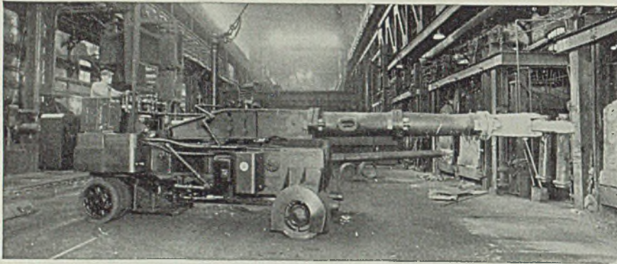
15,000 lb. Capacity Tongs Charger Serving Heating Furnaces and Steam Press.
