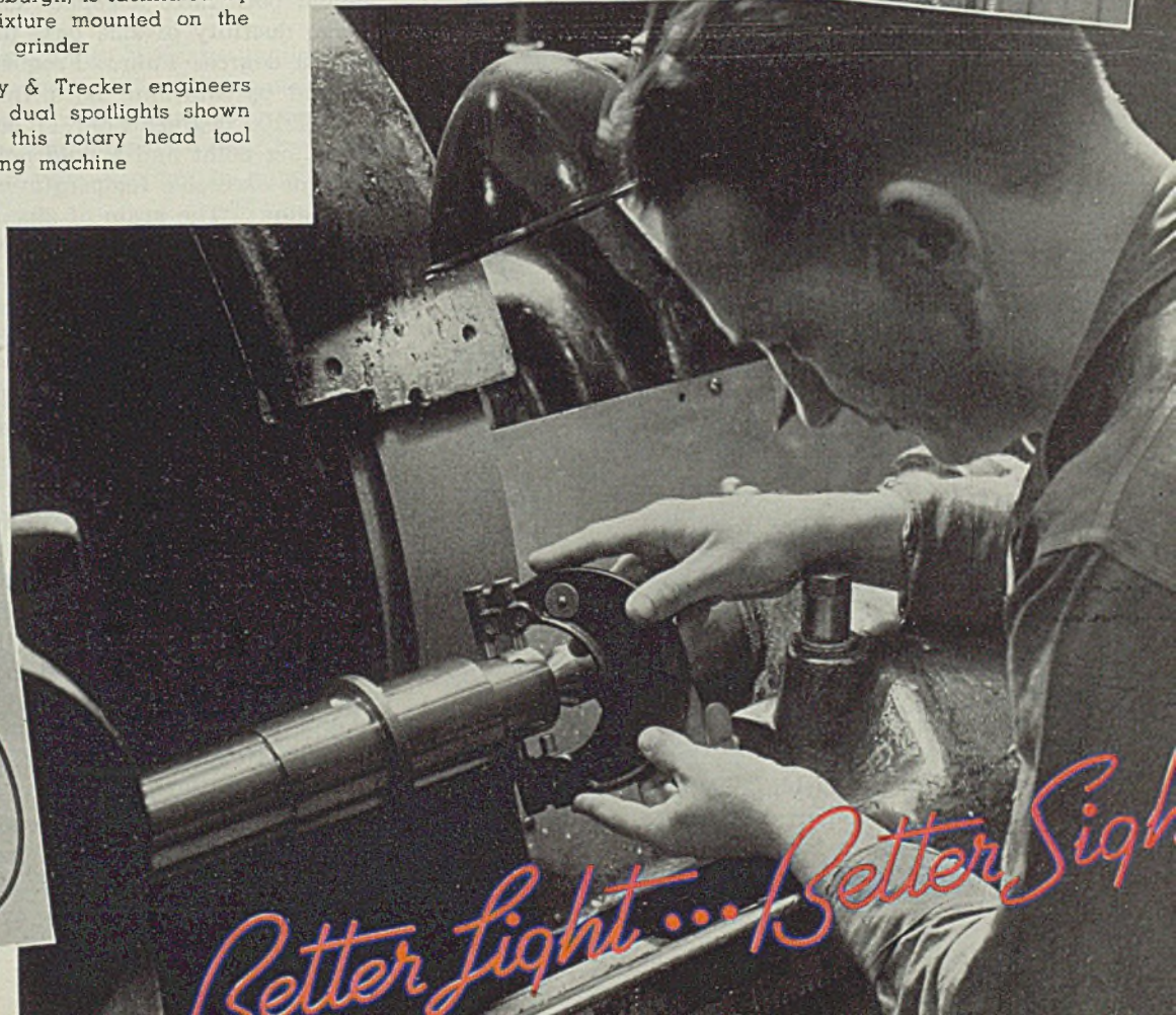
Fig. 2 (Center, below)—Taft-Peirce precision surface grinder has operation and "sighting" light housed behind translucent safety glass panel in guard
