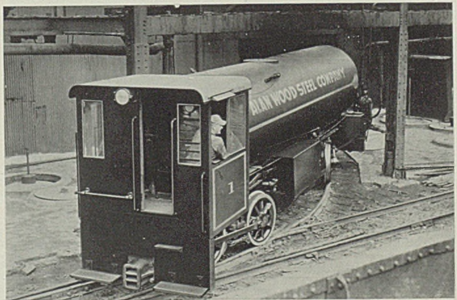
Fireless locomotive negotiating sharp curve at open-hearth shop located in Eastern Pennsylvania
