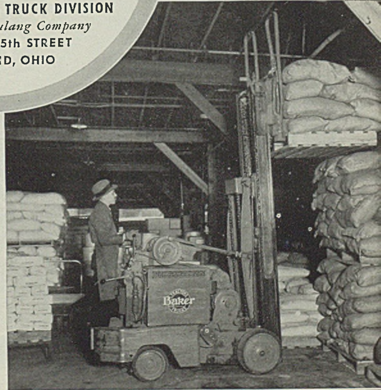
Tiering sacks of flour or sugar to the ceiling is a difficult job. Baker Tilting Telescoping Fork Trucks do it quickly, safely and efficiently in this large food warehouse.
