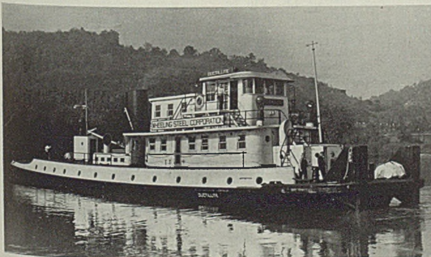
■ This 760-horsepower diesel towboat, the DUCTILLITE, recently was delivered to Wheeling Steel Corp., Wheeling, W. Va., by Dravo Corp., Pittsburgh. It is a new type of river towboat
