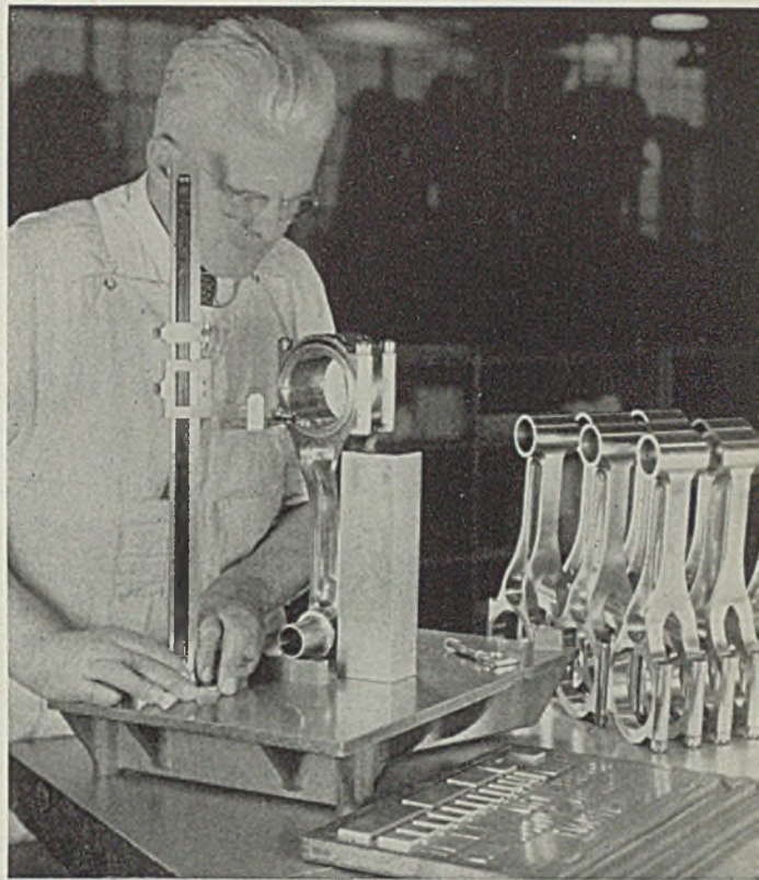
Fig. 4—To make sure that small and large holes are exactly parallel and exactly spaced, the assembled connecting rods are tested on a precision surface plate by means of a vernier height gage carrying a dial indicator
