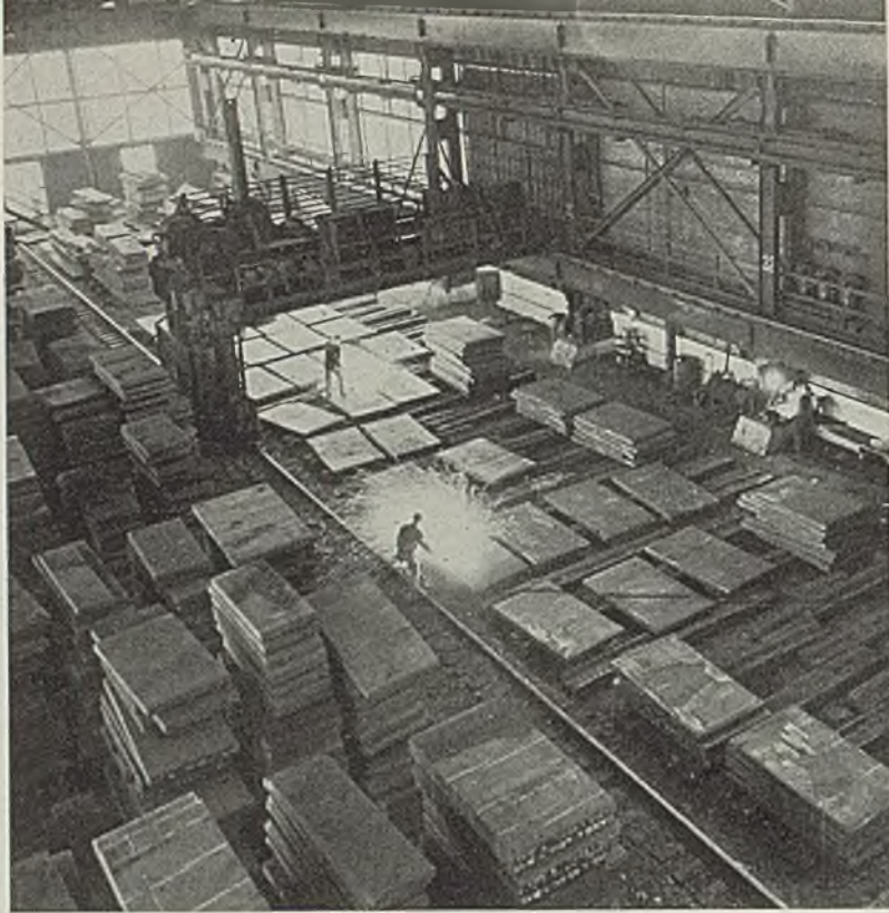
General view of strip mill slab yard showing scarfing beds and facilities provided for handling material
