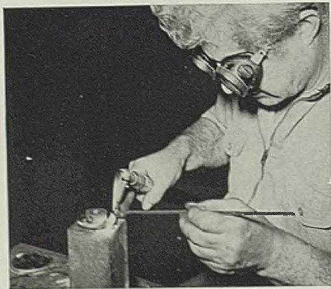
This worn cam is being rebuilt with cast iron for the seventh time. Illustrations courtesy The Linde Air Products Co., 30 East Forty-second street, New York
