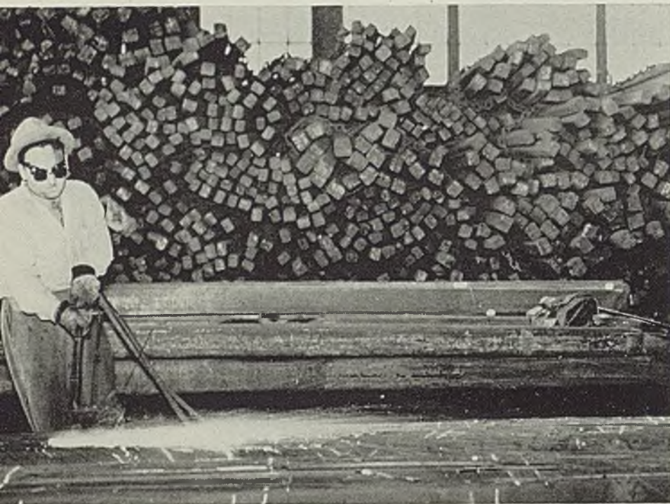
Scarfer conditioning the surface of billets
