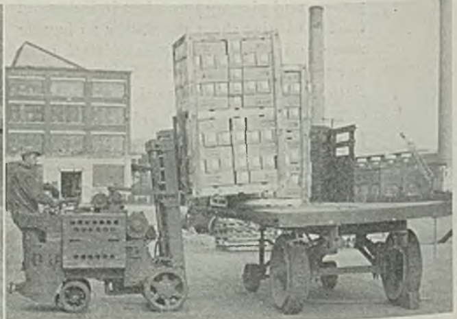
Fig. 3. (Left)—Here a 6000-pound capacity truck is enabled to handle easily an 8000-pound load by the use of a live skid taking part of the weight. Fig. 4. (Right)—Loading finished lightning arresters on a semi-trailer by means of a fork truck
