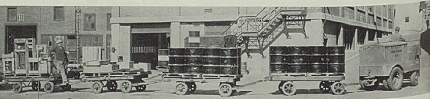
Fig. 1—Train of industrial tractor-trailer units handling loads on pallets
