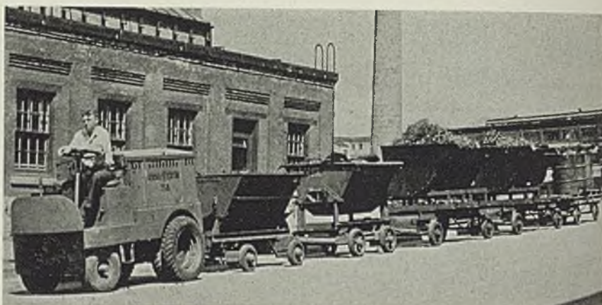
Fig. 11. (Left)—Removable dump body handled inside plant by fork truck. Fig. 12. (Right)—Tractor-trailer setup for handling salvage. Note dump hoppers on third and fourth trailers
