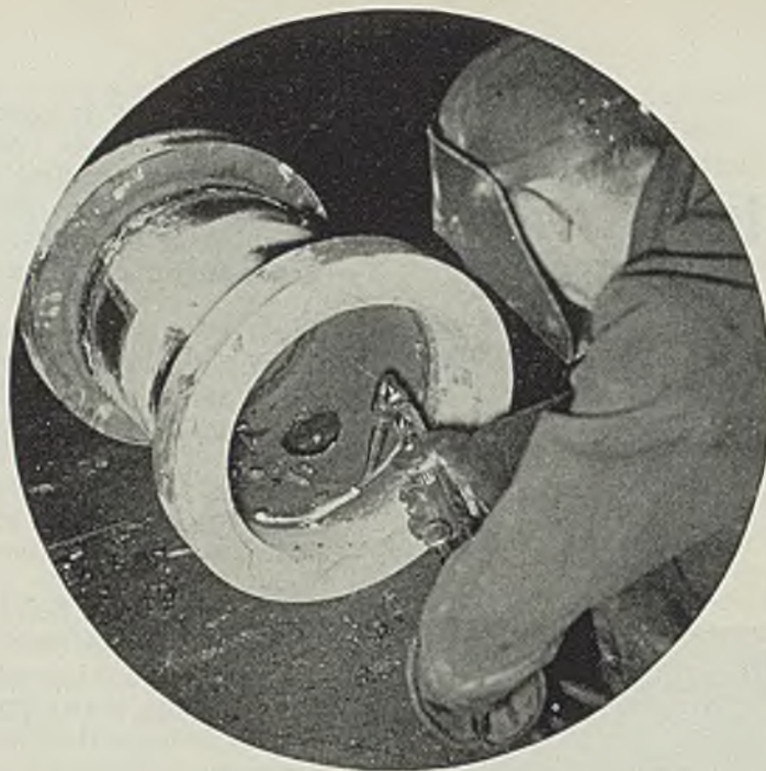
Fig. 1—An ordinary welding helmet protects the gouger from the hot gases and slag. Note the hand torch being used. Photos courtesy The Linde Air Products Co., New York
