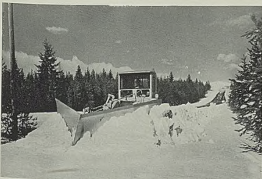
■ Familiar scene in many parts of the country: Diesel-powered, "motor grade" made by Caterpillar Tractor Co., Peoria, Ill. The V-shaped blade which forces snow to either side of the road is low-alloy, high tensile steel made by Republic Steel Corp., Cleveland
