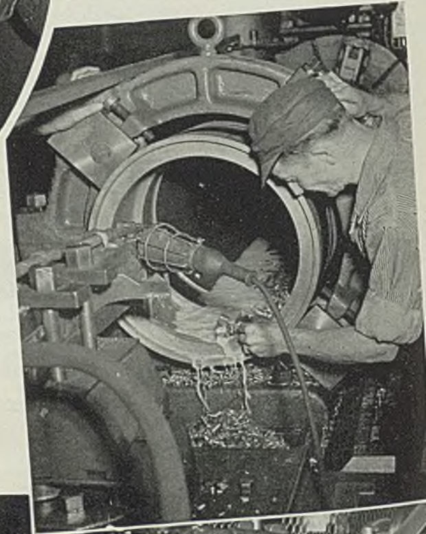
Fig. 1—Machining one of the forged steel end bulkheads, by means of tools held in turret tool post of a heavy-duty lathe. Contouring of the face, machining of the rim and boring of the hole already have been done. The hole is now being finished by a "floating" tool. Note the universal joint in its shank to provide the "float"
