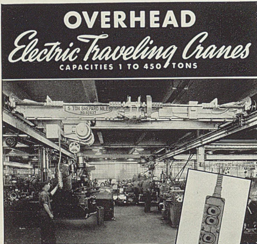
Selective 5-Speed Push Button Control applied to a Shepard Niles Inner-Running Trolley Crane.
