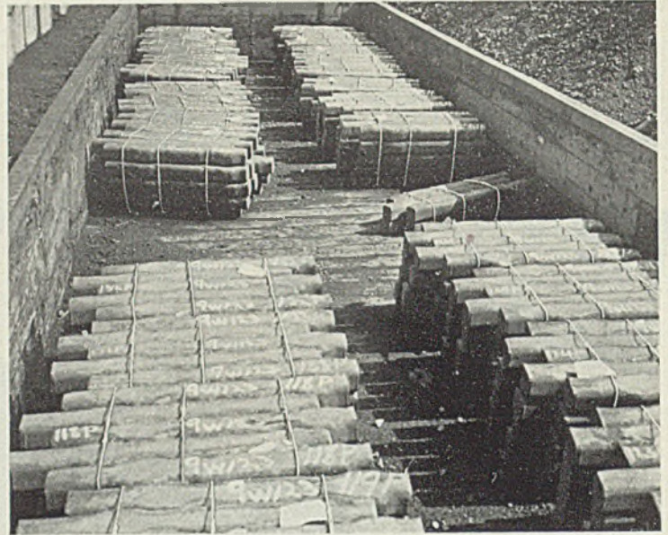
Fig. 1. (Left)—Heavy rough forgings wire strapped into bundles of 25 are easily picked up as a unit with a magnet crane. Fig. 2. (Right)—The crane quickly places the bundles in gondola cars. Thus handling is one simple operation from storage pile to freight car. Unloading is equally as simple
