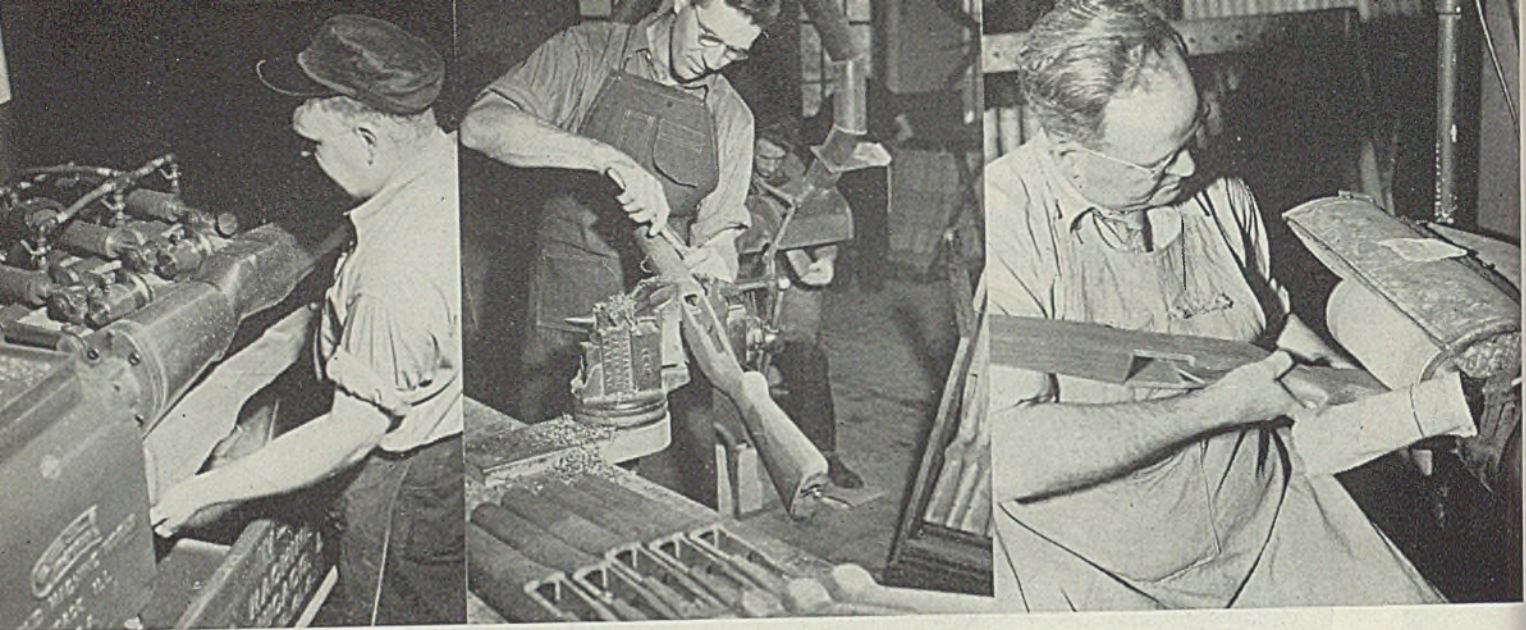
Figs. 7, 8 and 9—Turning rifle stocks on a copying machine, trimming by hand, and machine sanding for a fine finish, respectively. OEM photos by Palmer
