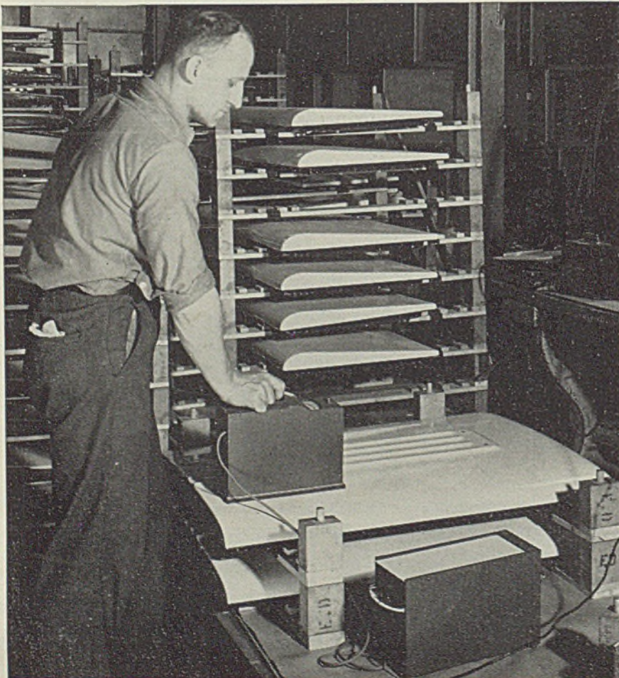
Fig. 2—Here the comparator is shown in use, placed on the surface to be compared. It affords a quick, accurate check on colors, making a more effective match than the human eye. Being entirely independent of the human equation, it is thus an important improvement
