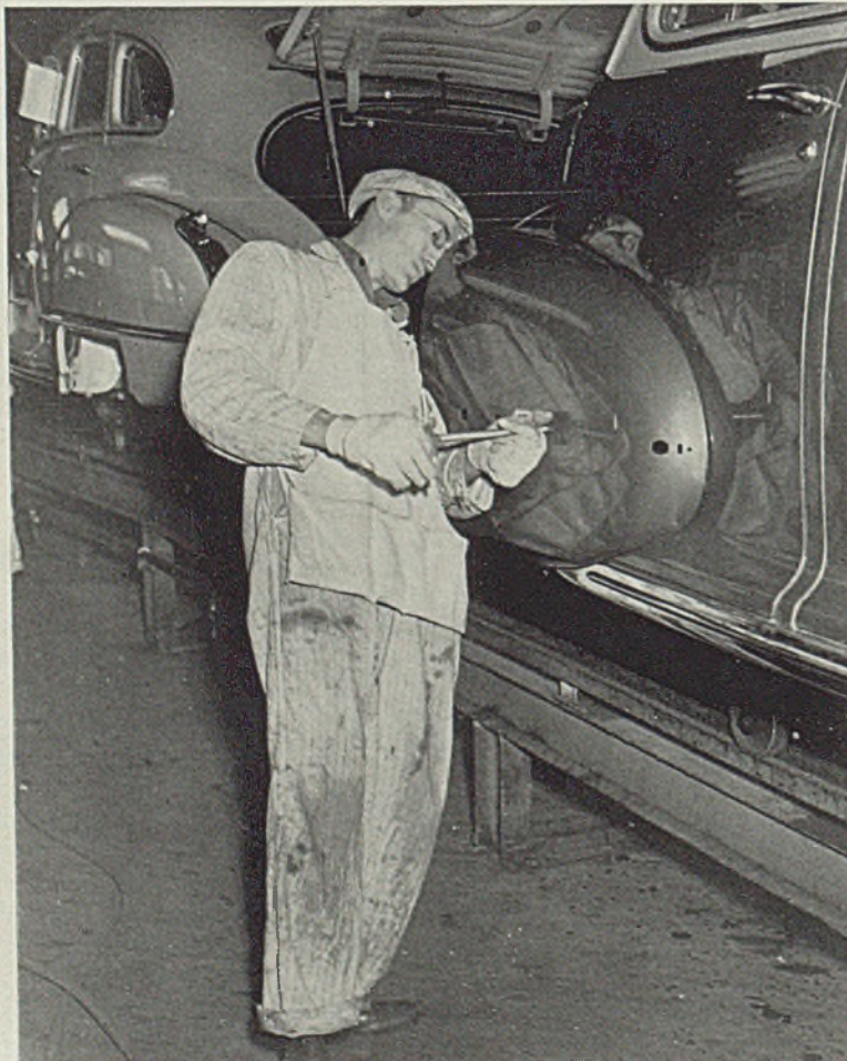
■ Placing the assembly line on stilts at the point where these fender caps are attached permits Cadillac workmen to stand erect while installing the cap on the door panel
