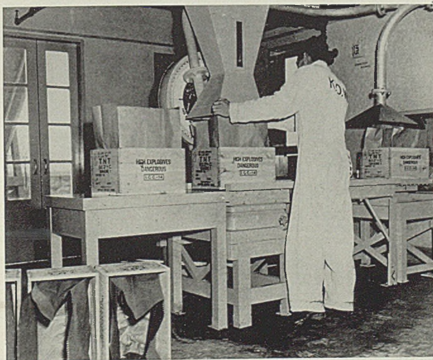
■ Filling paper-lined boxes with TNT in the "flaking house" of the Kankakee Ordnance Works, near Joliet, Ill., is expedited and made safe and easier for the operator by the handling system shown here. The box sets on a scale and 50 pounds of the explosive, flowing down the chute, is put into each container. Machine at the extreme right is a "vibrator", and shakes the TNT to box level. From this point the box is carried down a long, enclosed chute to the nailing house. NEA photo
