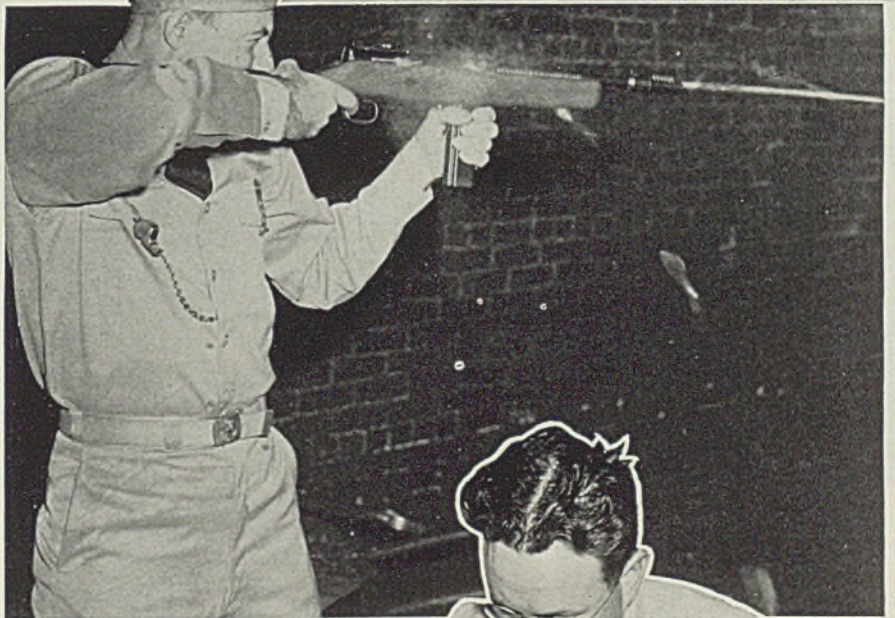
Fig. 1. (Top)—Extended view, fast firing Reising sub-machine gun. Specifications: Bottom fed, clips holding 20 cartridges; oil finish walnut stock, steel butt plate; firing rate, 450 to 500 shots per minute; weight 6.5 pounds; overall length, 35.25 inches; sight radius, 18.5 inches; fires .45-caliber bullets weighing 430 grains; penetrates 6 inches of white pine at 20 yards; bullet energy, 431 foot pounds; muzzle velocity, 920 feet per second
