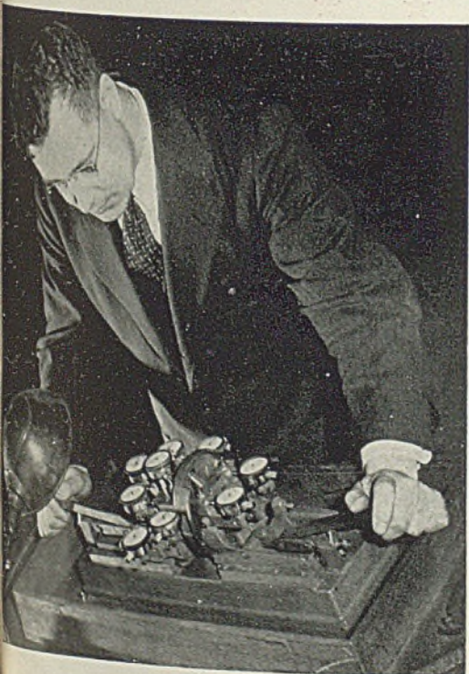
Fig. 4—Multiple-indicator gage allows operator to check simultaneously all critical dimensions of meter frames finished in the straight-line setup. Note double toggles to facilitate advancing the gages to working position
