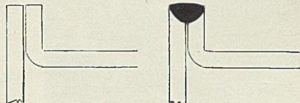
Fig. 9—Type of edge weld shown here is extremely economical as no filler metal is needed, yet a strong weld is produced
