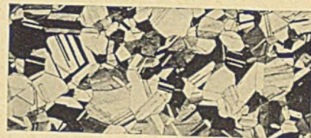
(Above) Annealed yellow brass, medium grain size, Mag. 75X. Tensile strength about 45,000 pounds per square inch.
