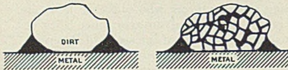
A solid dirt particle held on a metal surface by grease or oil.
