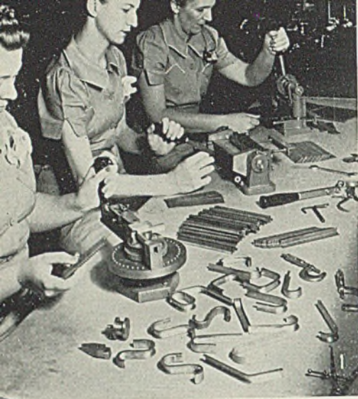
Fig. 1—Here is production setup of three machines shown in Figs. 2, 3 and 4 for producing formed channel sections
