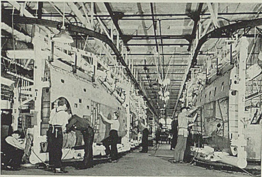
Wings travel in jigs around these two adjoining closed tracks, one for right and one for left wings, before being transferred to flat jigs for final installations and painting
