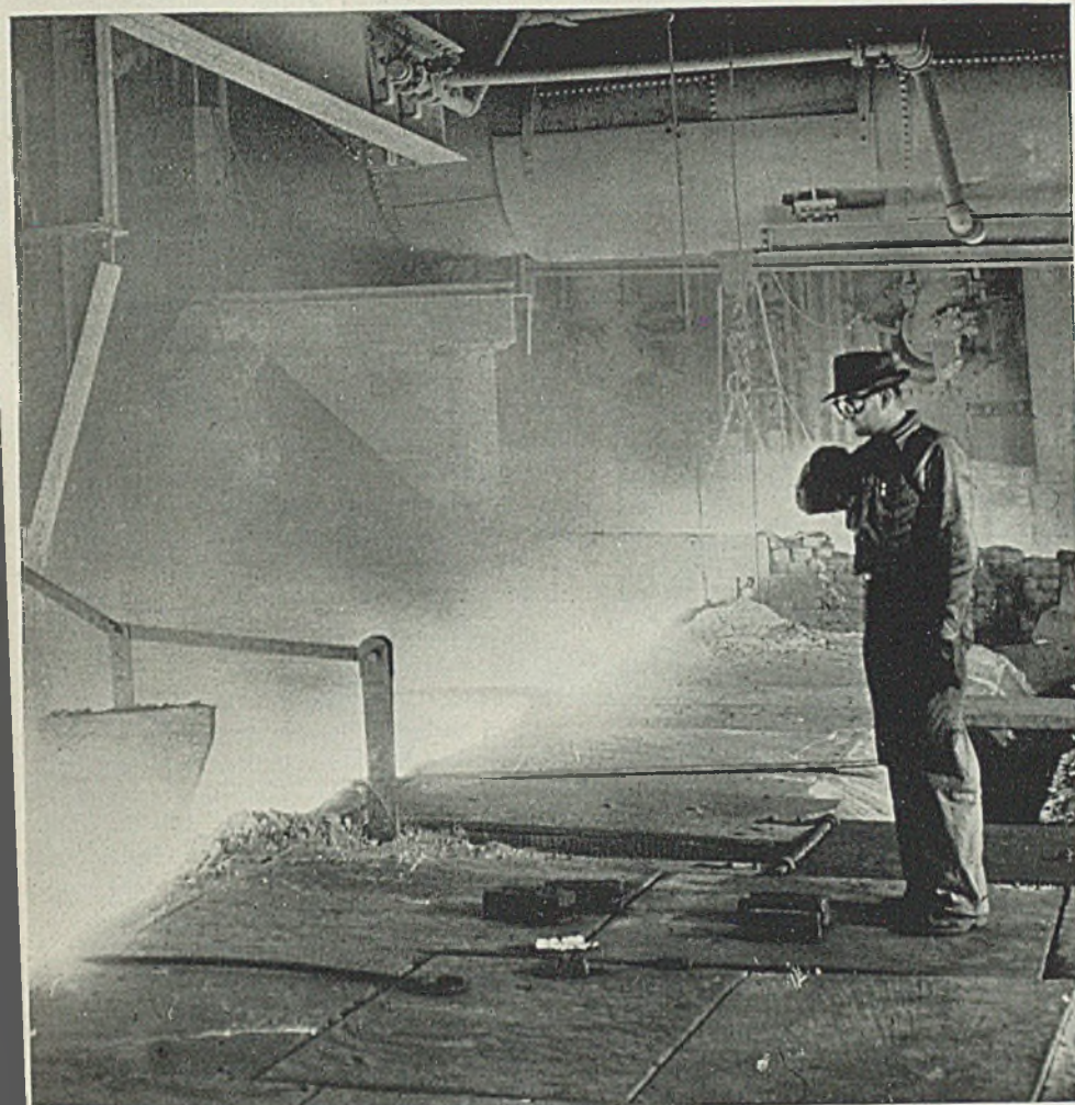
Thousands of tons of iron that had its inception in sinter flows down many runners of American blast furnaces today. Photo, U. S. Steel News
