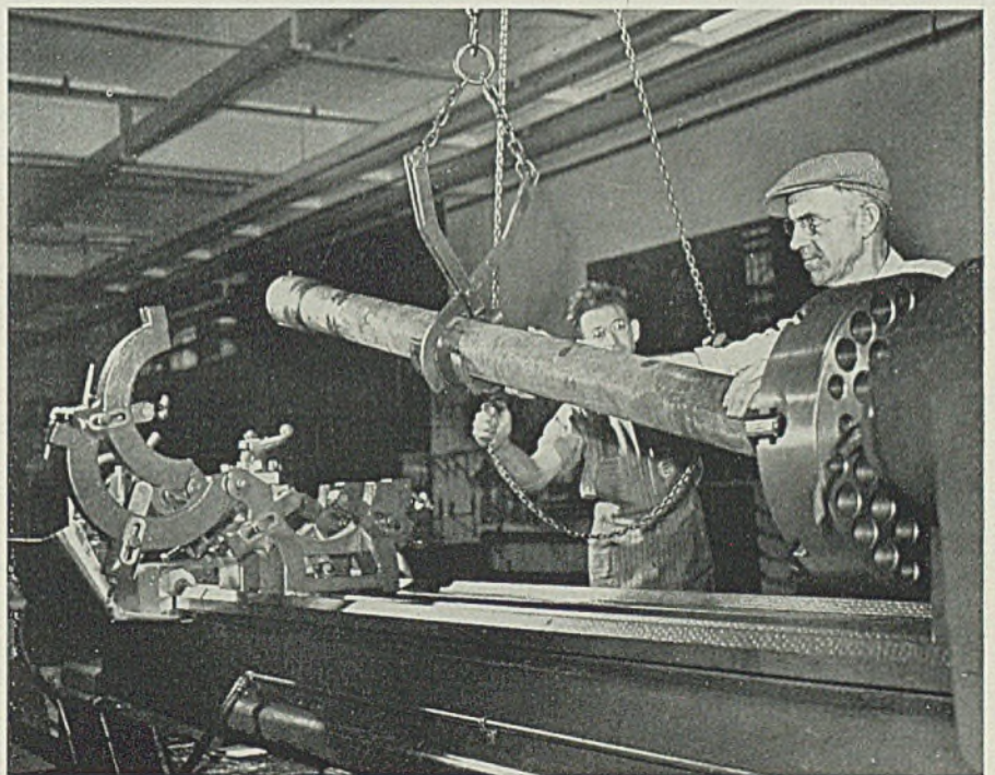
BARREL of the 40-millimeter field piece produced by Pontiac Motor Division starts out as a 443-pound forged steel blank, shown here as it is being chucked for the initial machining operation
