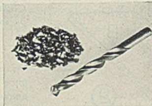
Tool used and chips produced in drilling free-machining Invar .
