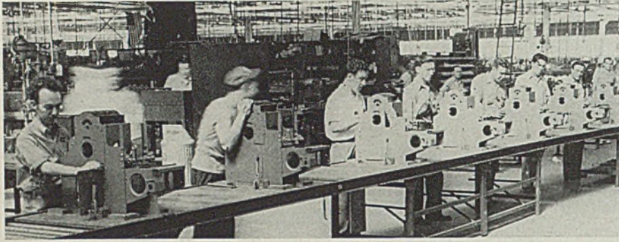
Fig. 5—Platforms with locating blocks and speed clamps are used with a roller conveyor to speed assembly of control pedestals here
