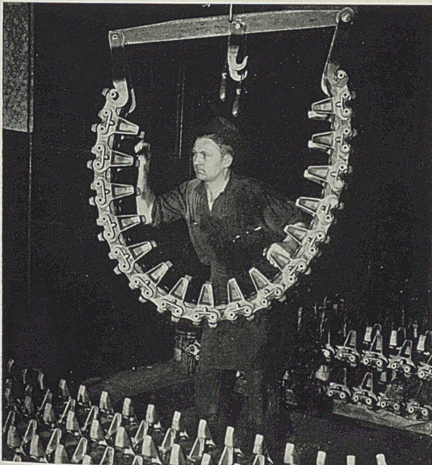
WRISTLET FOR HITLER! A workman tightens section of tank track and tread assembly in one of the buildings acquired from Hupp Motor Co. in Detroit by United States Rubber Co. The latter company required additional space to handle increasing tank track production
