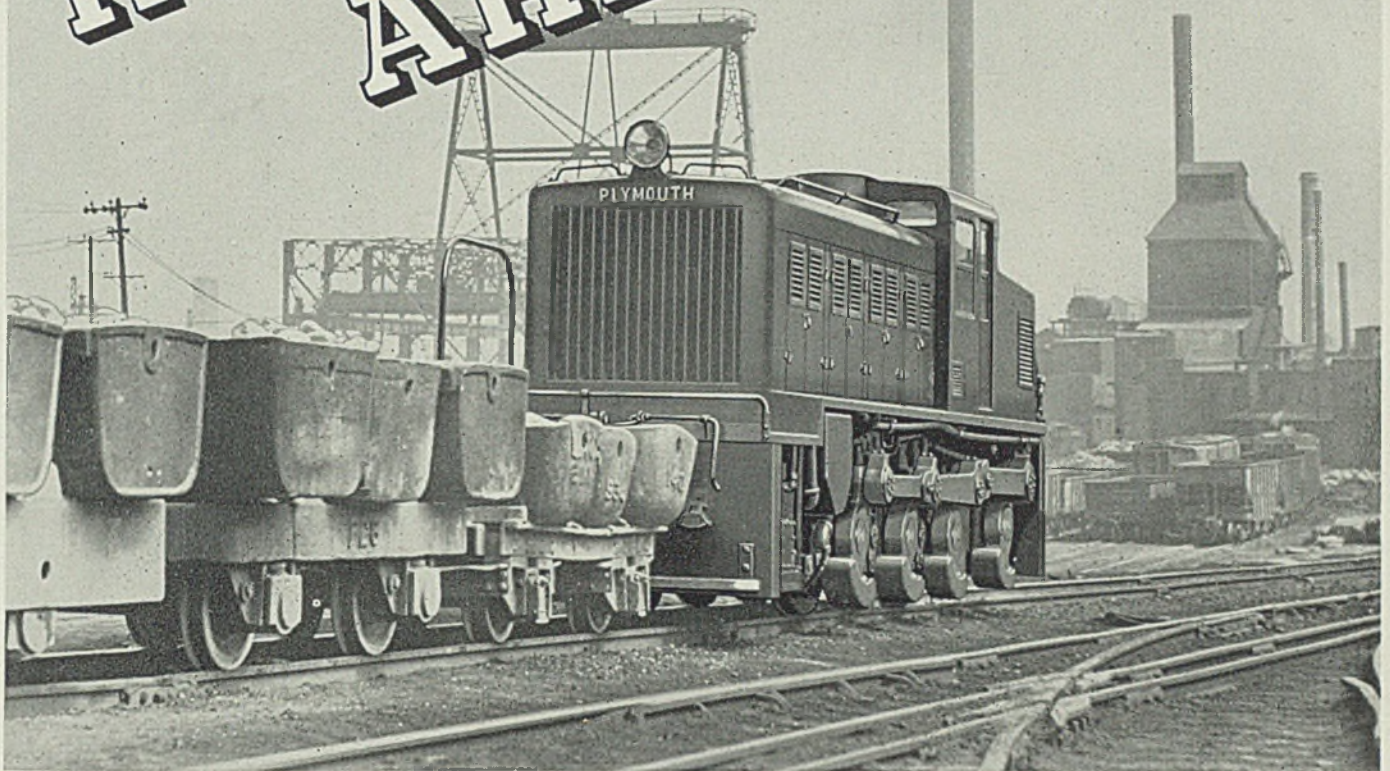
Plymouth 65-ton Diesel Flexmotive (mechanical drive) in operation in one of the country's outstanding steel mills.
