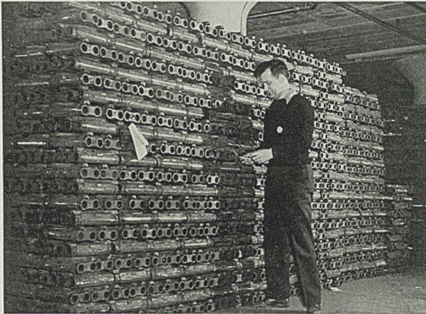
Large stocks of tank treads, which casual inspection reveals to be cast steel, awaiting assembly into tracks at plant of Hupp Motor Co. in Detroit leased by United States Rubber Co. to handle stepped-up program for supplying steel and rubber tracks for combat tanks
