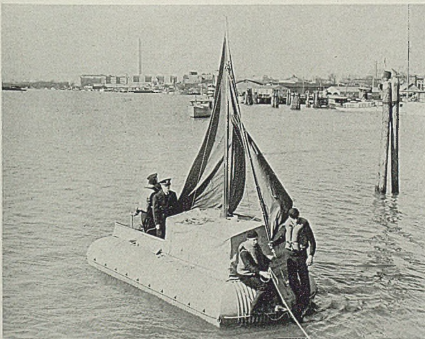
NEW steel life raft is demonstrated on the Potomac river in Washington. Approved by the United States Coast Guard, the steel rescue vessel may become standard equipment on merchant ships sailing into the war zones. It is designed to carry 20 men and is claimed to offer more safety and comfort than the life rafts now in use. NEA photo
