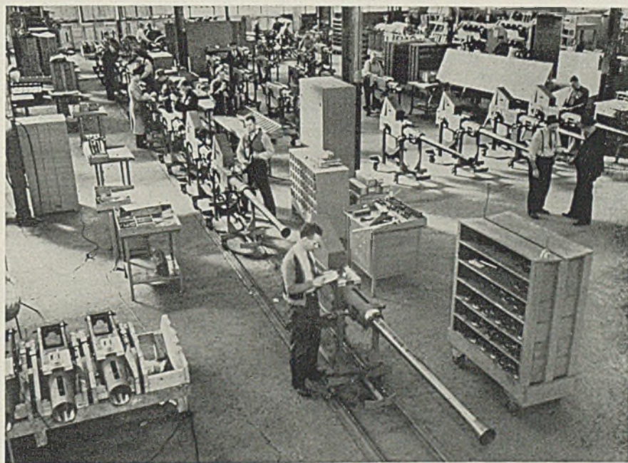
BOFORS-TYPE 40-millimeter field guns on the assembly line in a Pontiac Motor Division plant. Production of these weapons, along with 20-millimeter Oerlikon anti-aircraft cannon, makes Pontiac one of the largest producers of anti-aircraft equipment in the country
