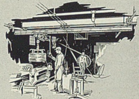
Stripping crane speeds up removal of wire coils.
