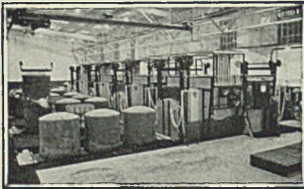
EF double ended electric furnaces nitriding aircraft engine parts.
