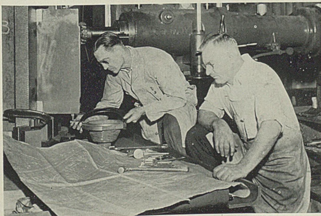
Initial tooling setups demand close co-operation between tool designers and tool-makers, inasmuch as the engineering drawings have to be translated directly by the machine tools rather than interpreted through jigs and fixtures as in production work. OEM Defense Photo by Palmer, courtesy Frederick Colman & Sons Inc., Detroit
