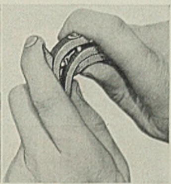
4. Bend belt further backward forcing enlarged opening down over rivet head until head is through.
