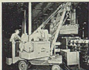
Small parts in standard boxes are tiered by Baker Truck to conserve space.
