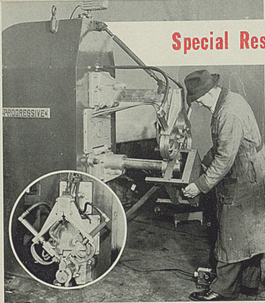
Fig. 1—Spot welding ordnance crates made from sheet metal. Two guns, each with two electrode tips, make four welds simultaneously under automatic control. Inset shows arrangement of electrodes
