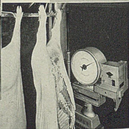
Fairbanks Portable Dial Scale with Printomatic weighing and printing records of meat to retailers.
