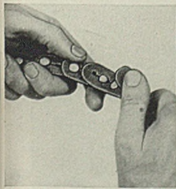
5. Straighten belt bringing rivet head up through enlarged hole.
