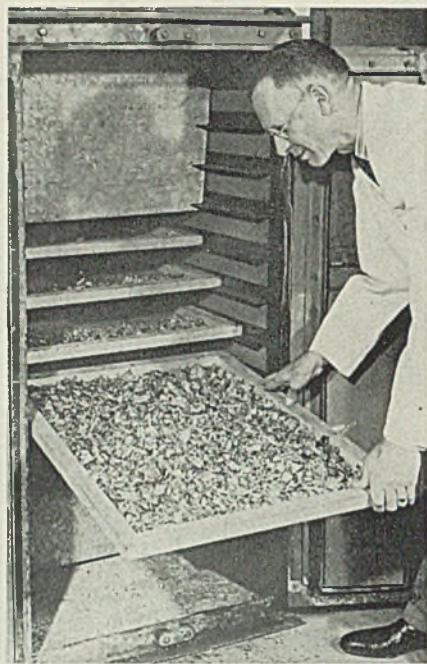
Ground raw meat as shown in the illustrations on preceding page subsequently is dehydrated in a cabinet drier wherein its moisture content is further reduced 10 per cent or less
