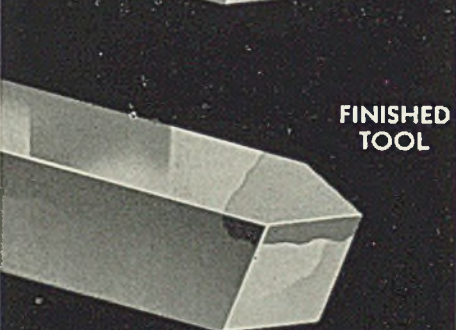
EFFICIENT CHISEL TIP FORMED BY ARC WELDING
