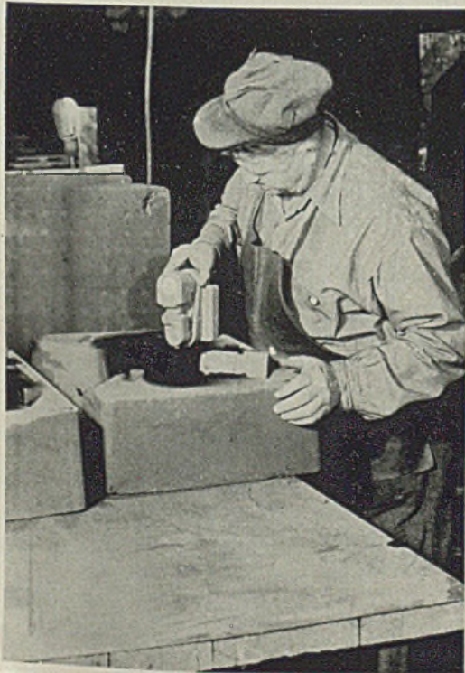
Fig. 10—Pouring test bars. Two test bars are poured from each heat
