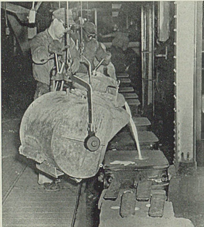
Steel at General Motors' Saginaw Malleable Iron Division is poured into quarter-ton covered teapot ladles, left, which are carried by electric hoist on an L-shaped monorail loop. A moving pouring floor is synchronized with endless type plate
