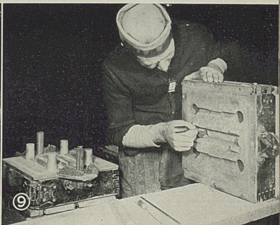
Fig. 10—Pouring test bars. Two test bars are poured from each heat
