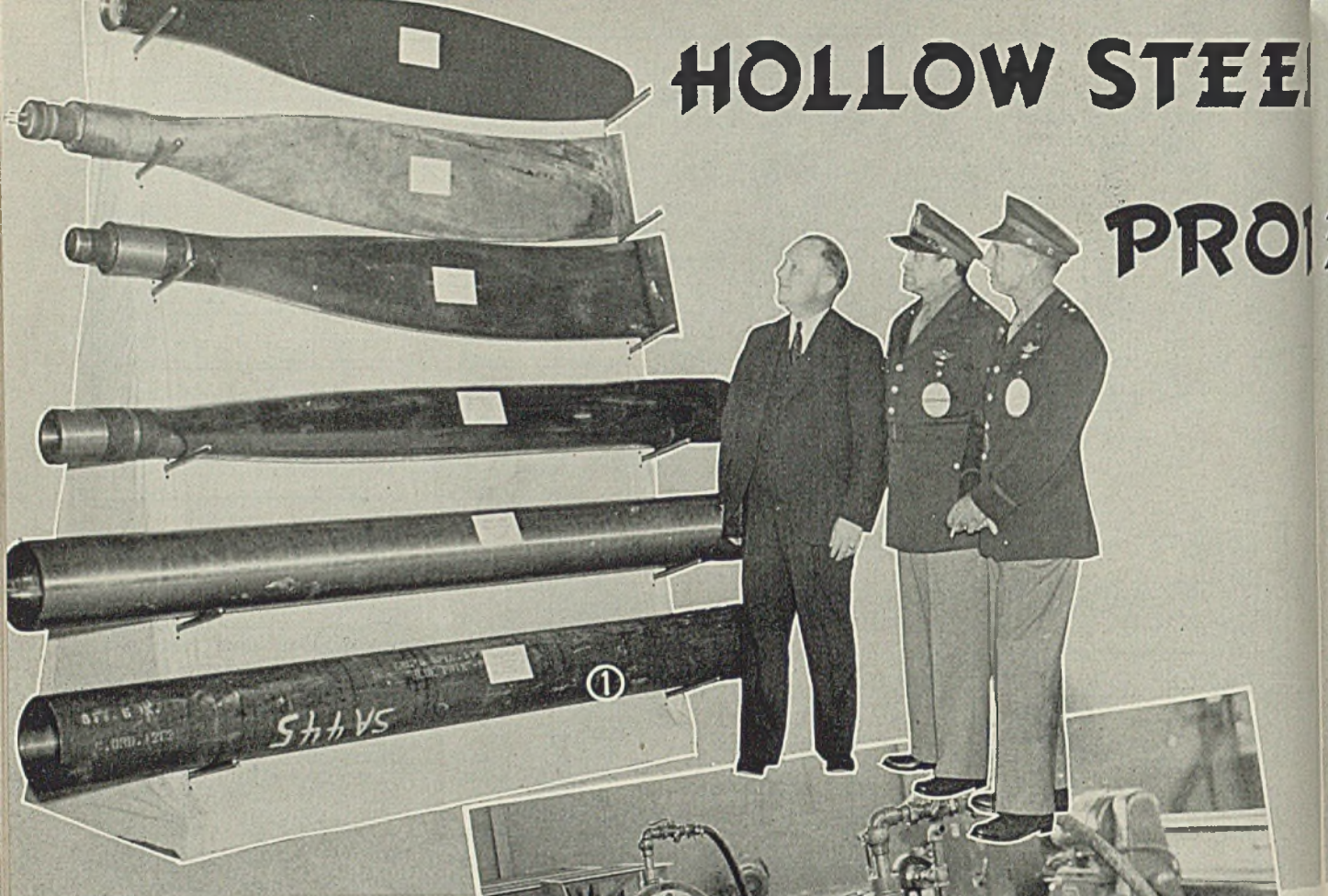
Fig. 1—E. M. Wise and Generals A. W. Vaniman and K. B. Wolfe of Army Air Forces observe various stages in manufacture of steel propeller blades
