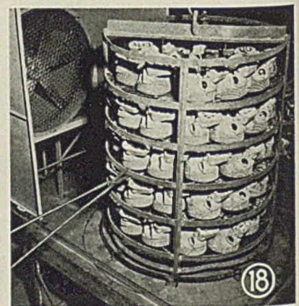
Fig. 18—Air quenching is done on this special setup employing a rotating table which revolves the loaded fixture in front of a powerful fan
