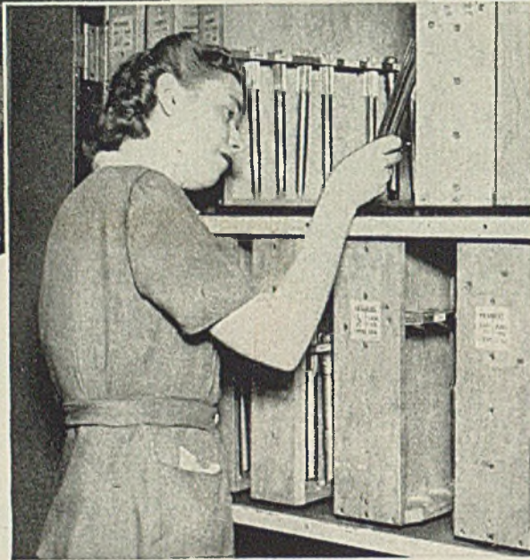
↑ Prominent numbering of the receptacles for small taps and plug and ring gages makes for speedy handling, minimum delay at the tool crib window in this efficient crib arrangement. Photo courtesy General Electric Co.
