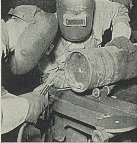
One-piece propeller blades are made from steel tubing. Page 93
