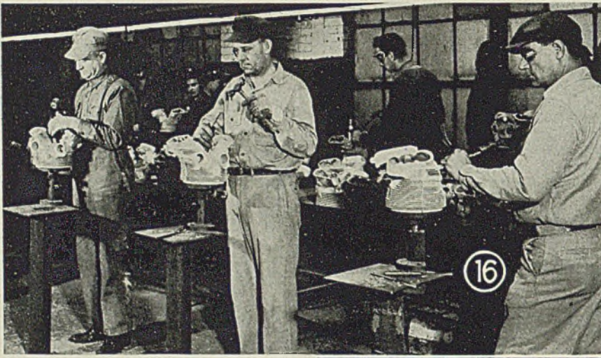
Fig. 16—Cleaning between the fins is a job that requires expert hand work—done on special stands shown here
