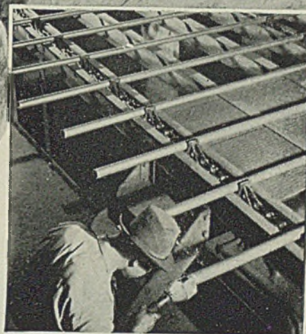
MORE SEAMLESS ALLOY STEEL TUBING to keep war equipment rolling off the production line. Construction with tubing instead of solid metal is one of the best ways to cut off dead weight and save steel.
