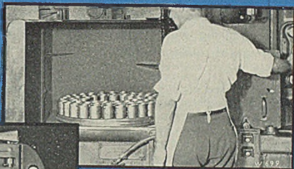
Grinding cylinder bushings on Blanchard No. 18 Surface Grinder
