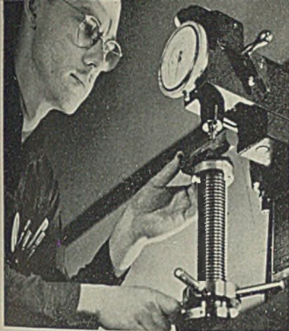
Jominy end-quench offers quick, simple test for hardenability of steel. Page 106
