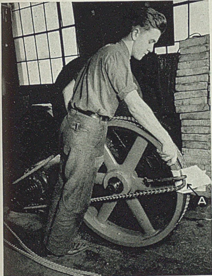
Position of correct length Veelos V-belt before drive is turned.
