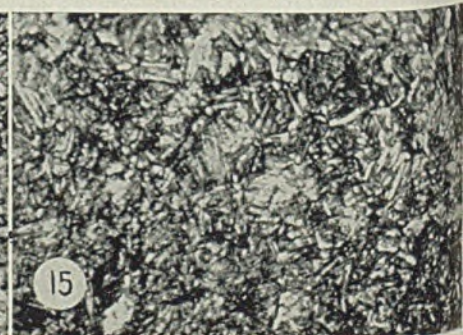
Fig. 13—Case structure of NE-9422 oil quenched from 1525 degrees Fahr. and drawn for 3 hours at 400 degrees Fahr. Shown at 750 diameters
