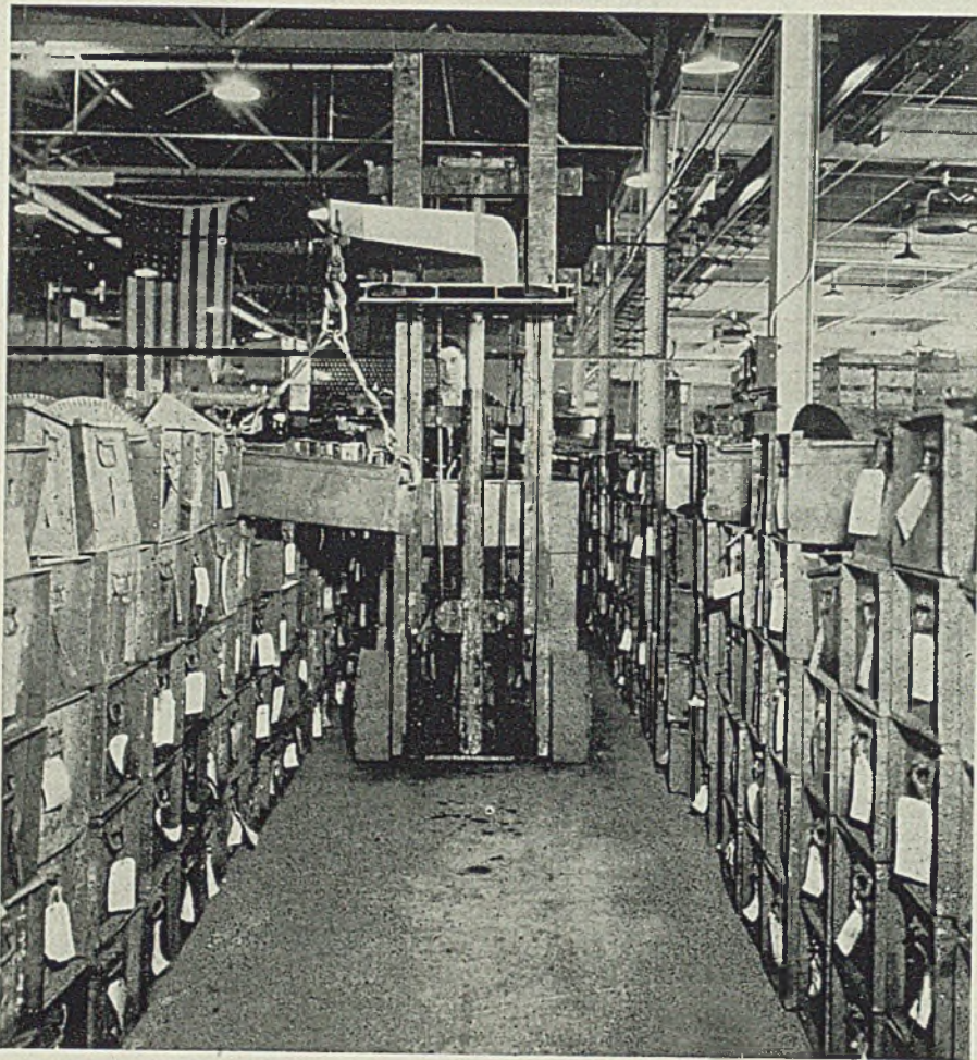
Fig. 4—Parts box being removed from bank by swing arm on fork truck in a narrow aisle
