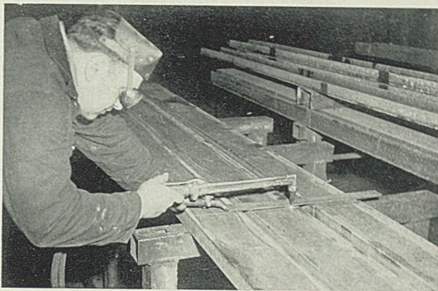
Fig. 11. (Below)—Laying out cuts like these involves use of accurate templets
