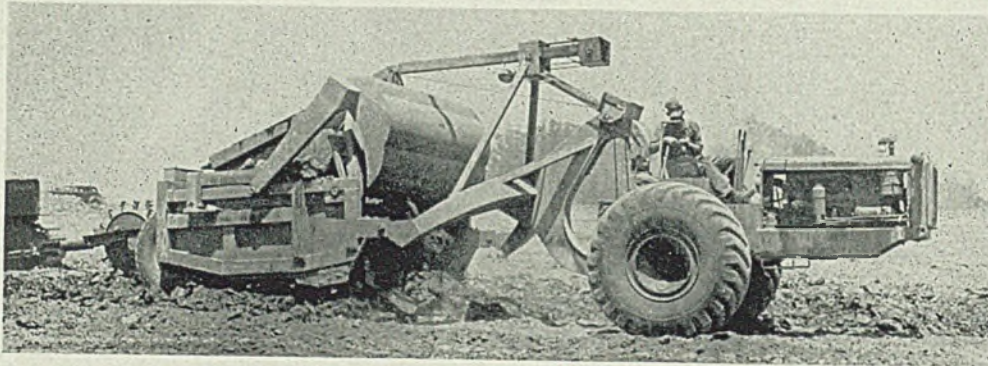
Fig. 6—In transition from experimental to mass production of a machine such as this, earthmover and tractor, careful checking of parts and their cutting templets is most important to avoid bad fits and costly welding
