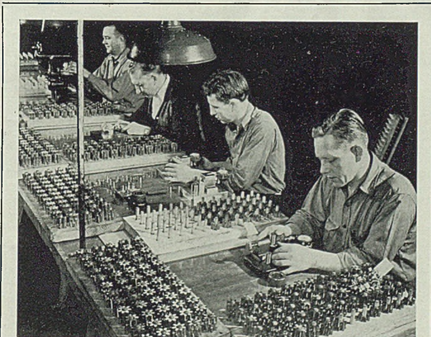
AIRCRAFT ENGINE GEARS: To avoid finger printing these precision finished aircraft engine gears and subsequent staining of the steel, these inspectors in a Chevrolet plant, building parts for Pratt & Whitney engines, use a special lotion on their fingers before handling the parts. Twelve distinct visual and physical inspections are required on these gears, finished to a tolerance of 0.0005-inch
