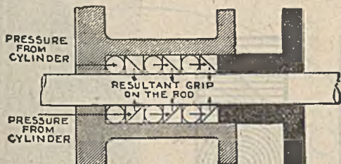
Fig. 33. —Principle of automatic diagonal packing. This packing does not depend on pressure from the gland, or on any expansion due to heat or due to the swelling of any substance, but does depend on pressure from the cylinder. This packing is an automatic packing commonly called "diagonal" packing, because it contains wedges which are formed by cutting a square section diagonally. There are a number of diagonal packings, differing from each other in the form and shape of wedges, but all of them depend upon the same fundamental principle that the pressure from within the cylinder will force the wedge next to the rod in toward the rod, and, of course, that means that the grip which it has on the rod will vary with the pressure forcing it, in other words, with the cylinder pressure.
