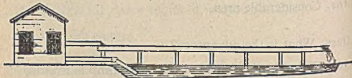
Figs. 1 and 2. —Non-directed flow natural cooling pond suitable for long and narrow lots.
