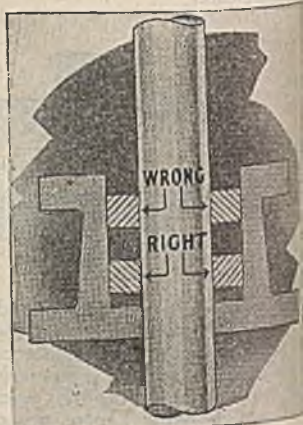
Figs. 34 to 36. —Typical sections of diagonal packing.
