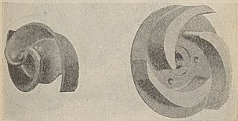
Fig. 7. —Two vane semi-open impeller with vanes designed especially for handling paper stock of high consistencies.
