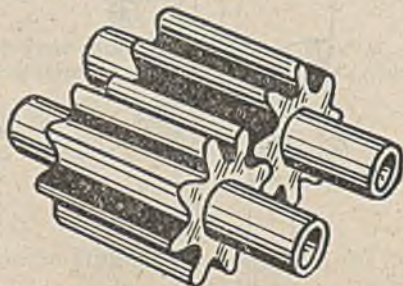
Fig. 8.—Gear Type Rotary Pumps 1: Spur gear rotary.
