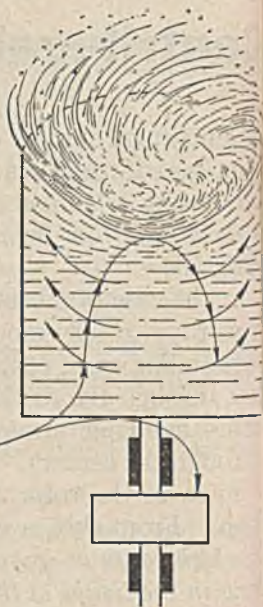
Figs. 1 and 2. —Cylindrical can with radial vanes illustrating centrifugal pump principles.
