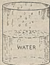
Figs. 22 to 24. —The three states of matter: solid, liquid and gas, as explained in the text. Note the first change of state from solid to liquid is called fusion and the second change of state from liquid to gas vaporization .
