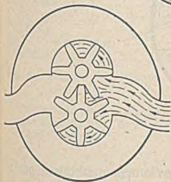
Figs. 2 to 4. —Operation of external spur gear pump. Fig. 2, liquid entering through admission opening; fig. 3, liquid being carried between the gear teeth toward discharge side; fig. 4, liquid being forced out of pump.
