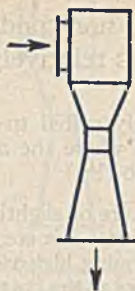
Fig. 5.—Single stage ejector. This type has a limited ratio of compression.
