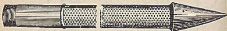
Fig. 6. —View of driven well point showing conical end and perforations through which water enters the pipe.
