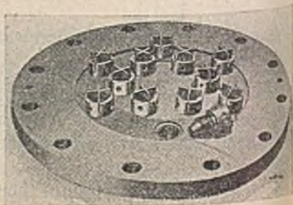
Fig. 17 .—Construction of nozzle plate and nozzles showing one nozzle removed. To accompany fig. 16.
