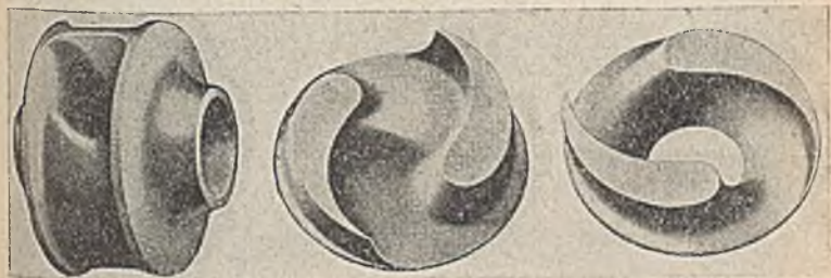
Figs. 41 to 43.—Impeller for handling trash. Fig. 41, general appearance; figs. 42 and 43, same impeller sawed in half to show more clearly shape of vanes.
