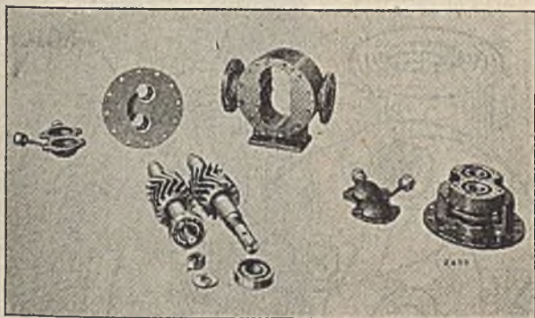
Figs. 19 to 24.—Gear Type Rotary Pumps 6: Disassembly view of double helical gear pump with external ball bearings.
