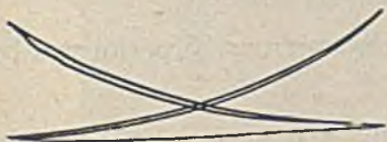
Figs. 25 to 34. —Indicator diagrams showing operation of clearance control at five load points.
