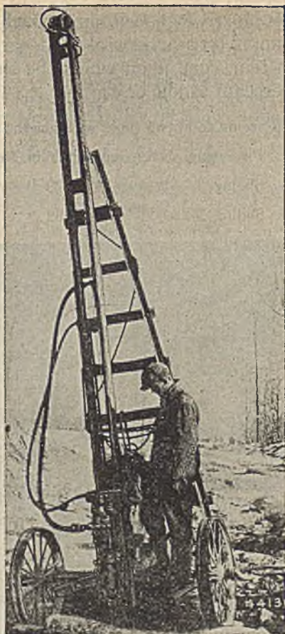
Fig. 11. —Wagon mounted jackhammer—a one-man outfit. Useful on many road construction jobs, in foundation work for bridges, buildings, dams, etc., and in certain phases of quarry work. By means of a self-locking worm drive a small, four cylinder air motor automatically feeds the drill up to the rock exactly as with a hand cranked drill. This method prevents the drill jumping back, thus eliminating the use of unnecessary feed pressure which causes rotation binding. It also prevents the drill dropping on the operator, and keeps the drill from jumping forward in a soft spot or when a steel breaks. This self-locking feature also protects the air motor from thrust and shock.
