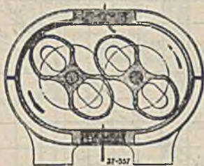
FIG. 2.—Root positive displacement super-charger. Inside the casing are two gears mounted on two shafts, one driving the other. In the blower chamber attached to these shafts are two double rotors set at an angle of 90^\circ with each other.
