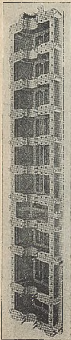
Fig. 50. —Bed plate for the frame shown in fig. 49. Note provision for the multi-throw crank.
