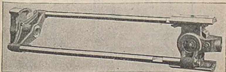
Figs. 19 and 20. —Straight line double cross head and tow rod construction with detail of the power cross head for the unit shown in figs. 16 to 18.
