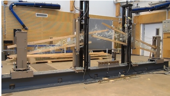
Figure 5.5: Four-point bending test of life-size hybrid beam with web made of heat-strengthened glass.
