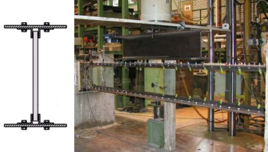
Figure 2.7: Cross-section of the hybrid steel-glass beam and four-point bending test [26].
