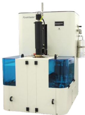
Rys. 116. Porozymetr Pore Master 60 firmy Quantachrome Corporation.
